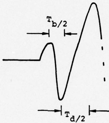
Figure 3.2.1 Sketch of a typical explosion P-wave with dominant period measurements,  $T_b$  and  $T_d$ , indicated.
