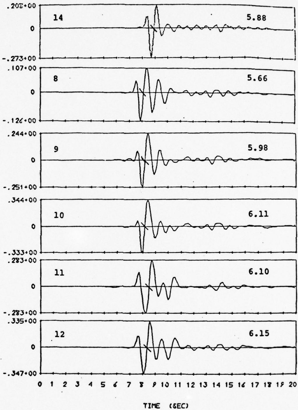
Figure 3.1.10. Synthetic short period seismograms for one spherically symmetric and five cratering calculations in wet sandstone. The numbers to the left are ground motion in microns at 1 Hz.
