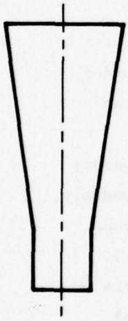
(a) STRAIGHT WALL, STRAIGHT CENTERLINE
