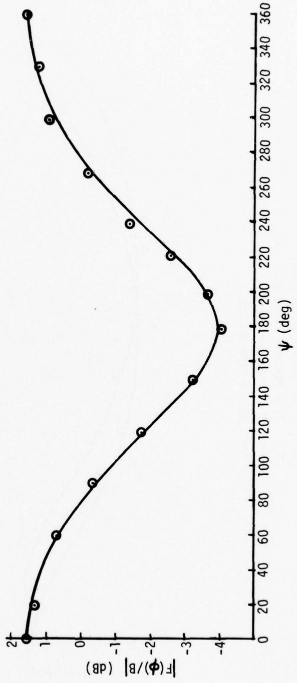
Figure 4. 72 Hz Comparison of Measured Data With New WTF Pattern Factor for Casco, Maine (0 dB = -144.35 dBA/m,  $\Delta \sim 0^\circ$ )
