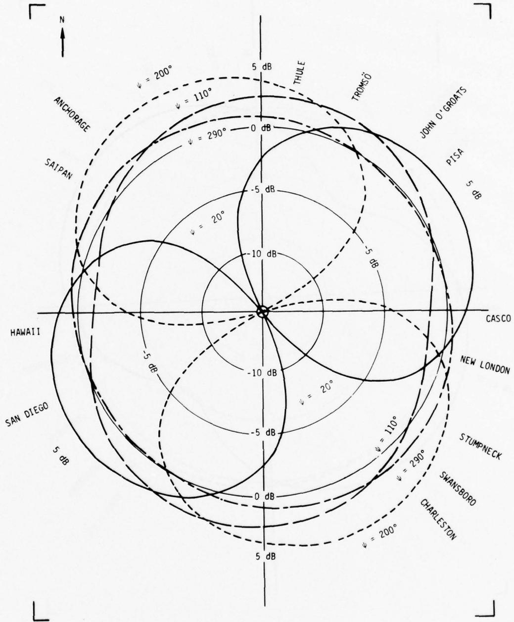
Figure 9. 70 to 80 Hz Band New WTF Pattern Factor Versus Receiving Location Bearing;  $\psi = 20^\circ, 110^\circ, 200^\circ, \text{ and } 290^\circ$
