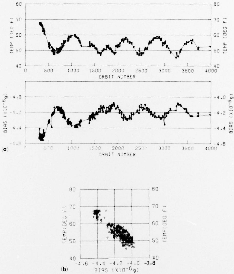
Figure 4. Orbital Bias Results Obtained With the AE-E YX Sensor. (a) Orbital bias data vs sensor temperature and orbit number; and (b) scatter diagram of bias vs sensor temperature
