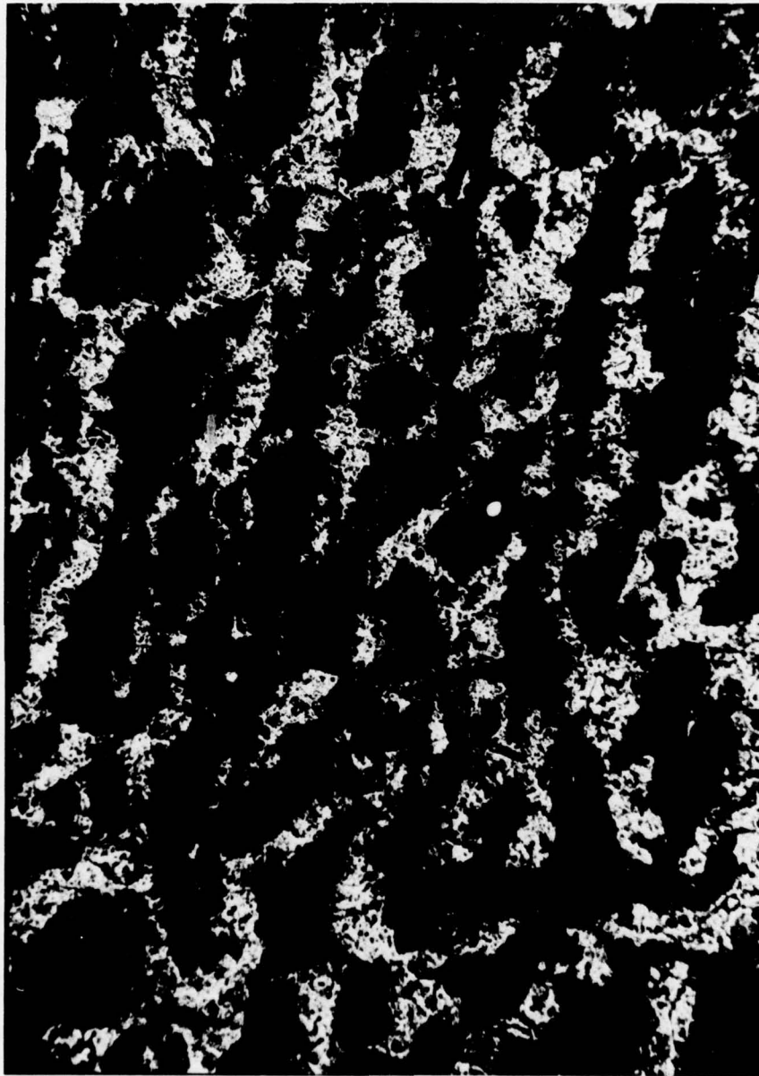
Figure 36. Magnification of 28× of a vertical thin section of the Toledo Penn 7 material after freezing
