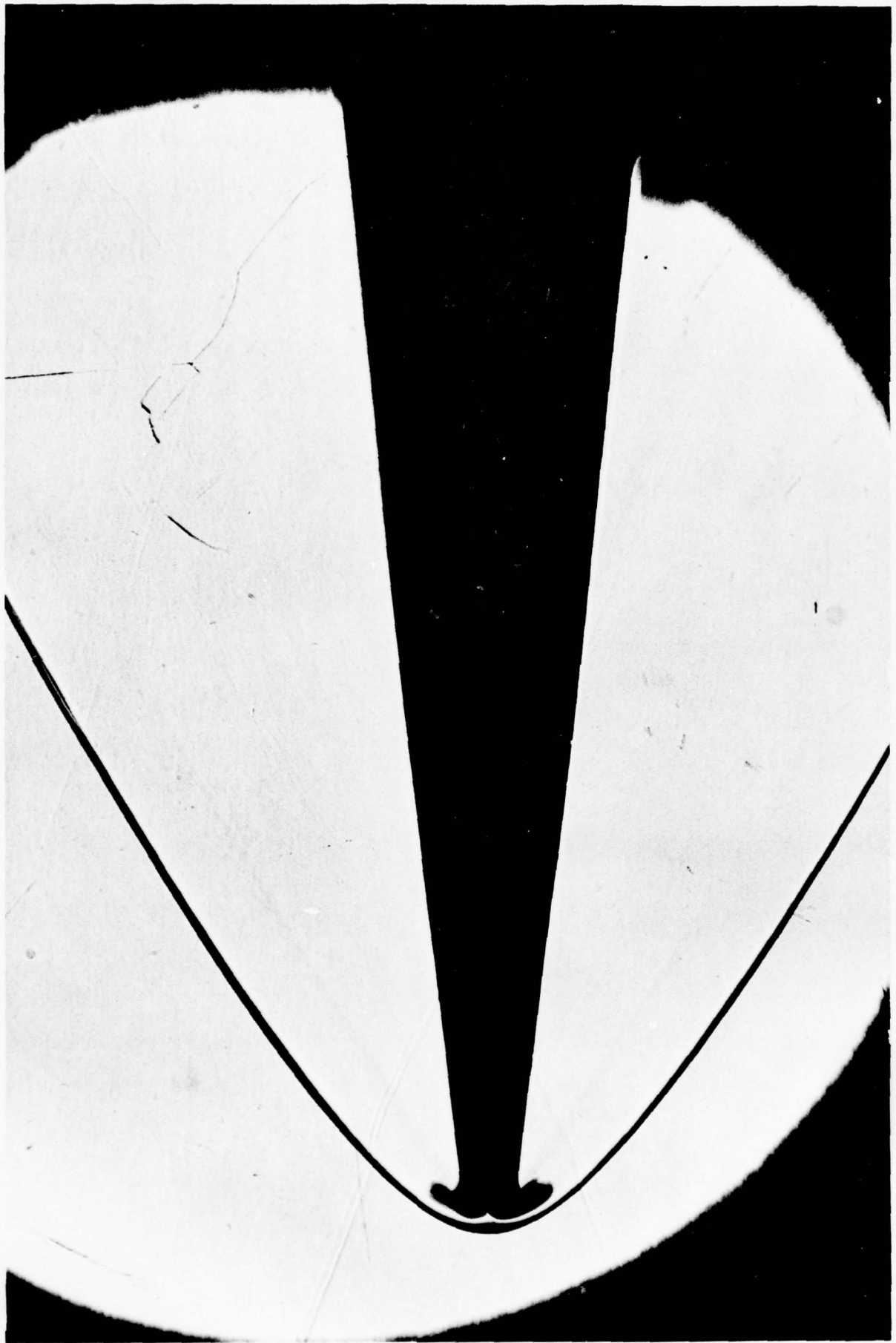
Figure 8. Shadow Photograph of Shock Shape for D = .635\text{cm} (.250\text{in}) , \alpha_G = 6^\circ .
