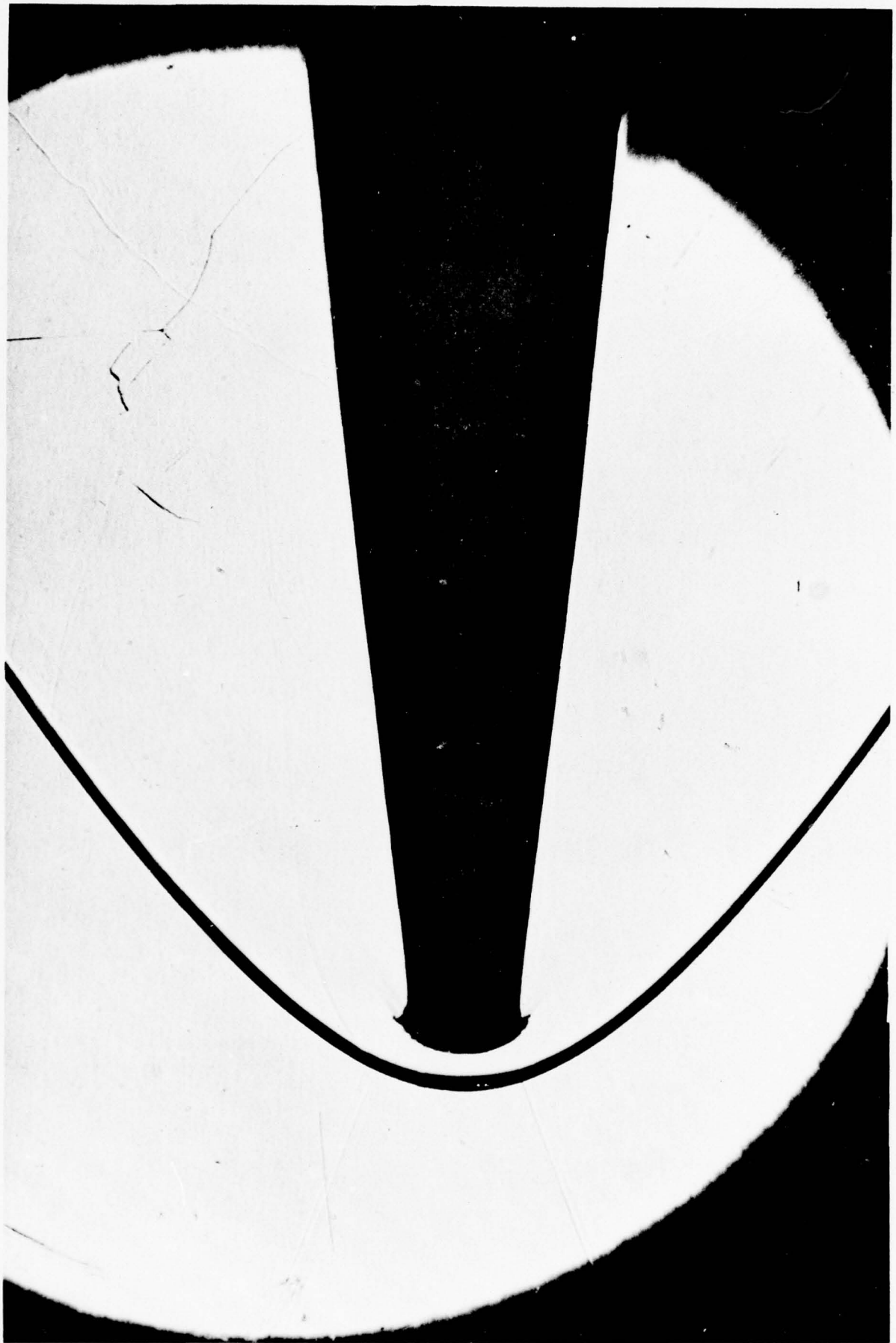
Figure 9. Shadow Photograph of Shock Shape for D = 1.27\text{cm} (.500\text{")} , \alpha_G = 6^\circ .
