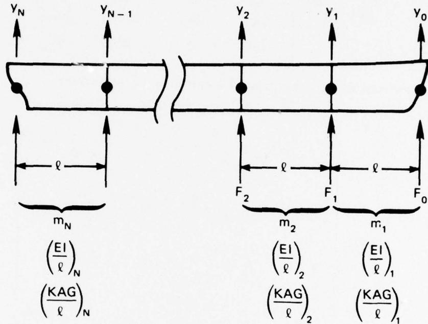
Figure 1 – Structural Model for Vertical Vibration of a Ship Hull
