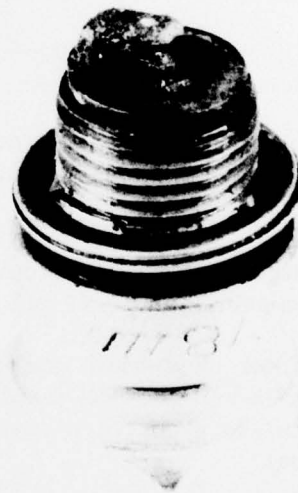
(b) Test 18: MIL-L-22851B, Type III Oil (AL-6534-L) 100 hours 16:1 fuel/oil ratio 265° CHT @ 7,000 RPM 77.6 Merit Rating 4 Fouled Plugs
