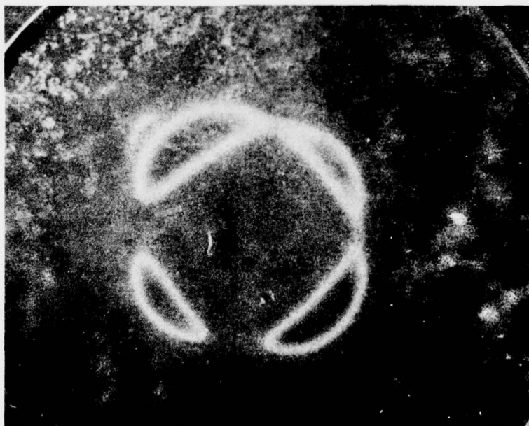
Figure 4. First Higher Order Mode Structure on Disc Antenna With Feed 0.56 cm From Center (4.7 GHz). (a) Calculated; and (b) observed
