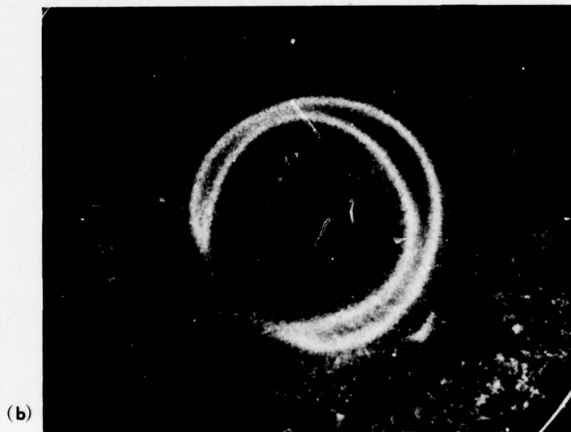
Figure 5. Second Higher Order Mode Structure on Disc Antenna With Feed 0.56 cm From Center (6.5 GHz). (a) Calculated; and (b) observed
