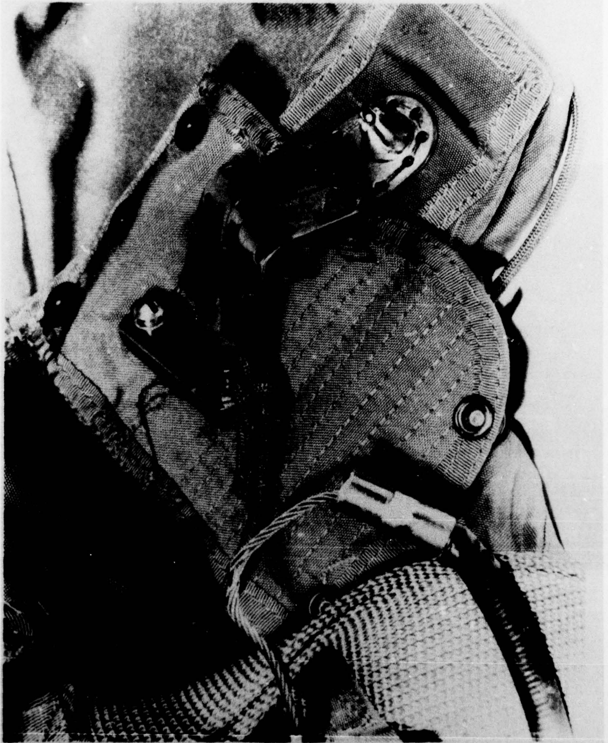
FIGURE 14 - Alameda Clamp and Bracket - After Test No. 3.
