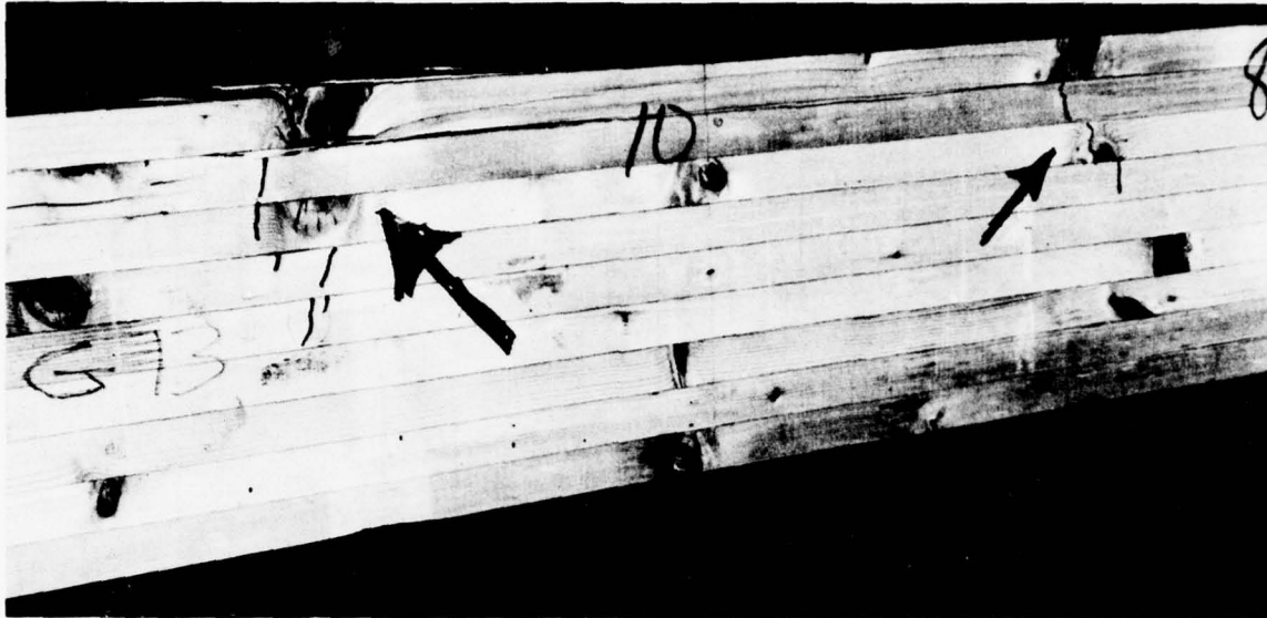
Figure 7.—Compression failures occurred throughout the top one-half of beam G-13 at two locations within the highly stressed region. Large knots in the top and third-from-top laminations were involved near both the 9- and 11-ft locations. Load was applied at the 8- and 12-ft locations. A total of 10 beams developed significant compression wrinkles; the other 9 were generally limited to the top 2 or 3 laminations.
