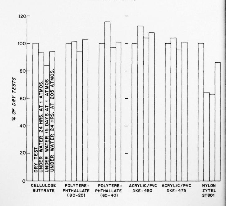
Increasing hydrostatic pressure from one atmosphere to 205 atmospheres for a period of 24 hours did not result in more rapid loss of cut and stab resistance by any of the plastics.
