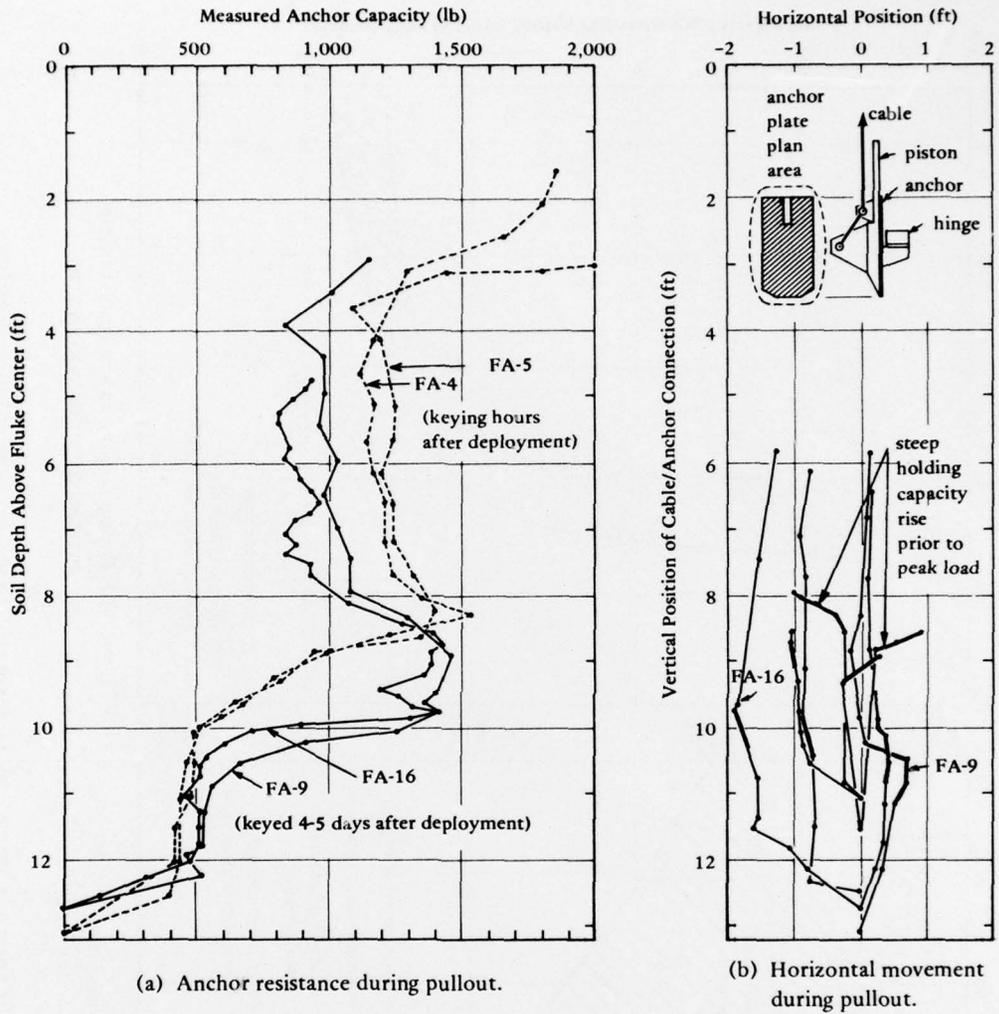
Figure 7. Vertical and horizontal anchor movements during pullout.
