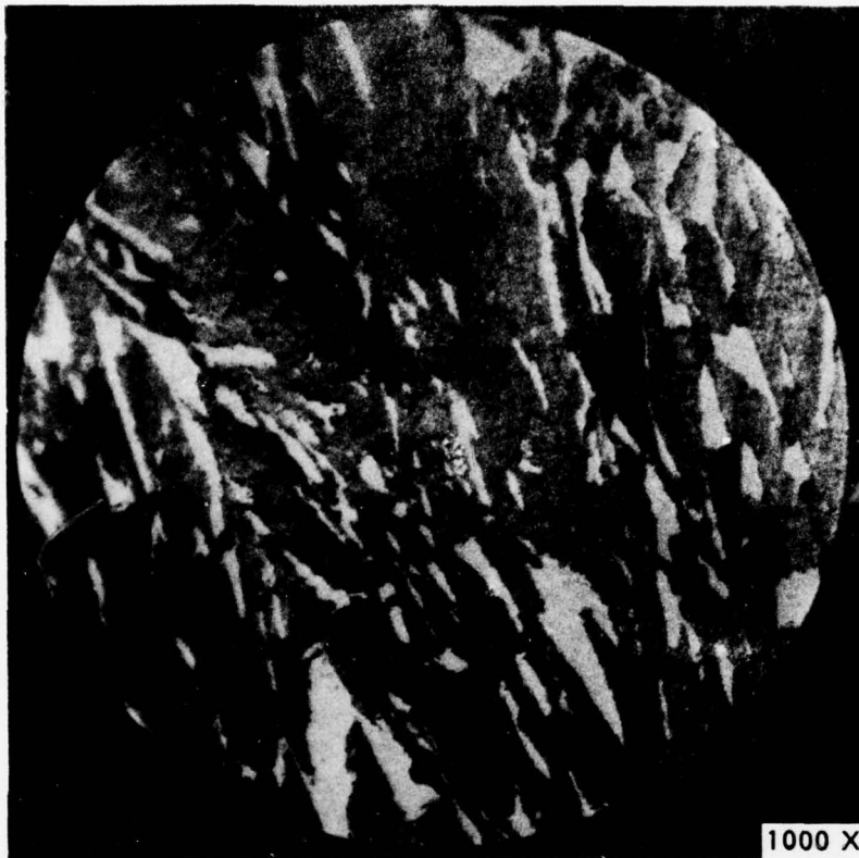
Figure 93. Typical Group 30 PG/SiC Microstructure.
