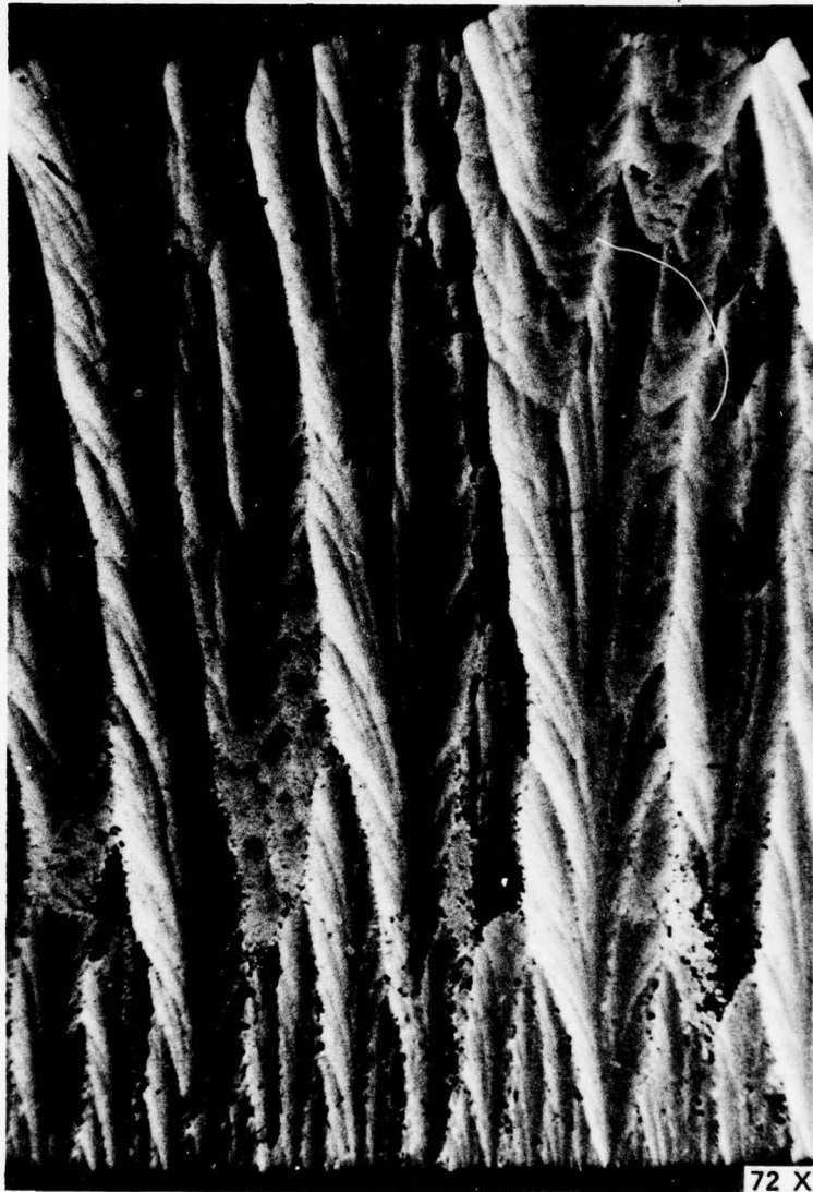
Figure 57. Run 008-11, Entrance End, Coating Microstructure (Full Thickness).
