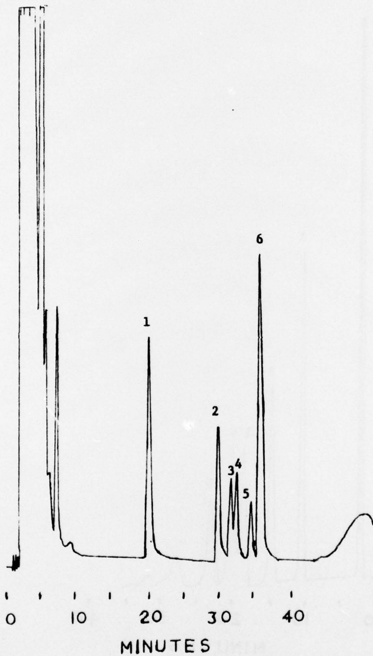
Figure 3. Determination of aromatics in the known solvent using the proposed method. Peaks: 1, toluene; 2, ethylbenzene; 3, para-xylene; 4, meta-xylene; 5, ortho-xylene; 6, internal standard (cumene).
