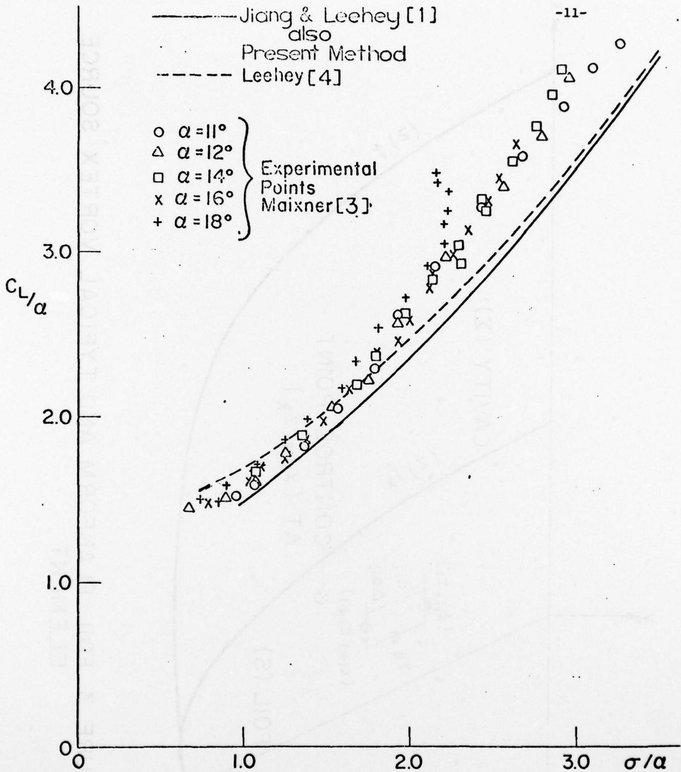
FIGURE 4 Lift Coefficient of Elliptical Planform, Aspect Ratio 5.
