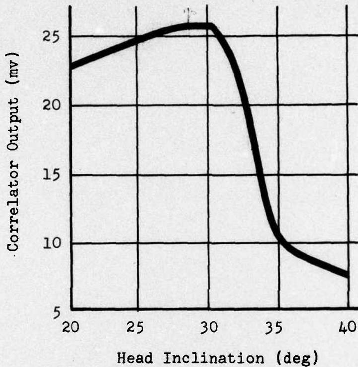
Figure 8. Variation of Response of Correlator with Inclination Angle of Record Head
