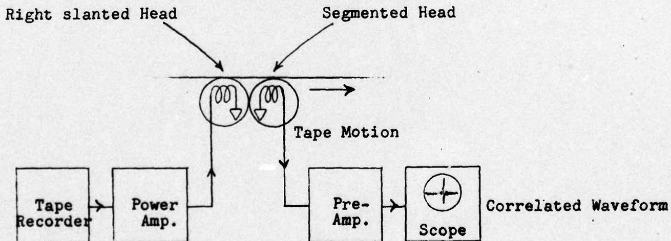
1(b) Obtaining compressed pulse from correlation waveform
