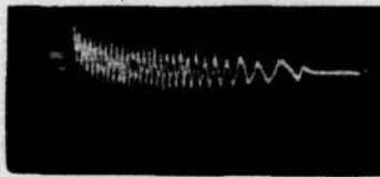
Figure 6. Electronically Generated Correlating Waveform
