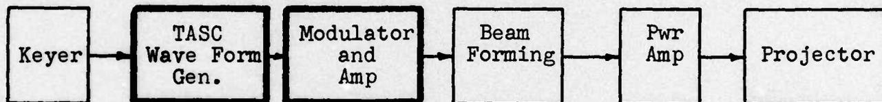
2(a) Sonar Transmitter transmits the TASC waveform.
