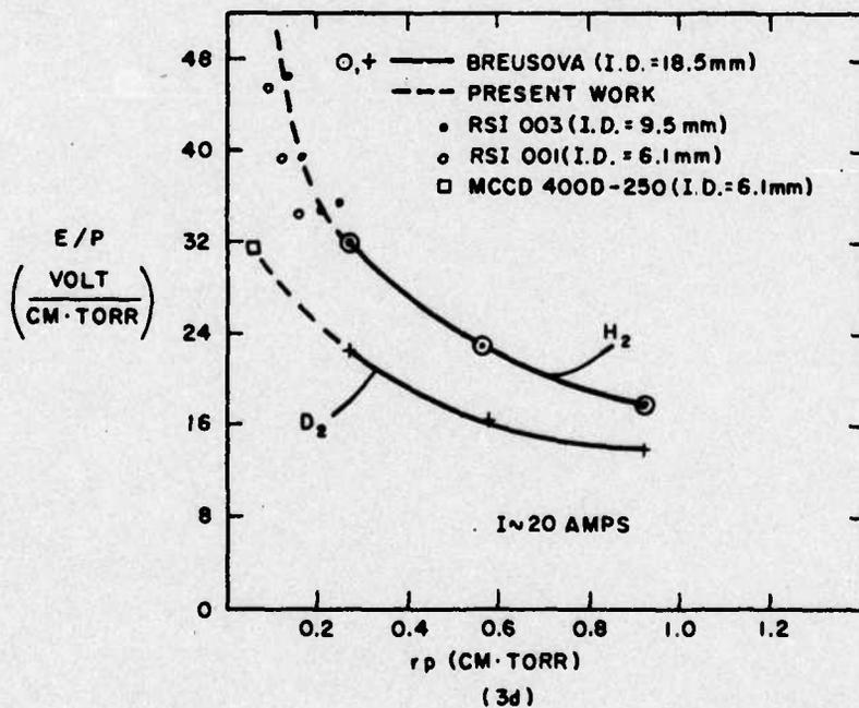
Figure 3. Voltage drop vs. current and pressure: comparison of results.
