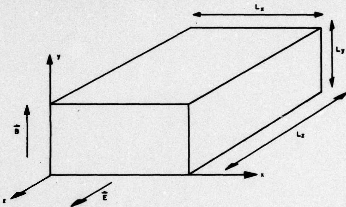
Figure 13. Geometry for positive column analysis.
