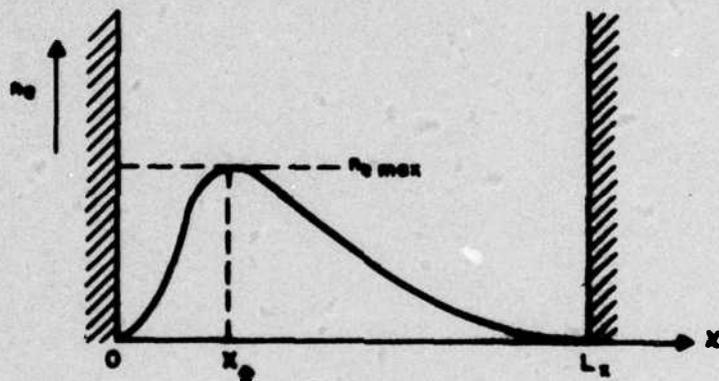
Figure 14. Solution form for electron density vs.  $x$  for a positive column in a transverse magnetic field.
