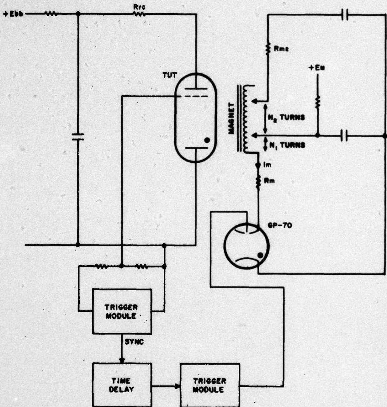
Figure 9. Magnetic field shaping test circuit.
