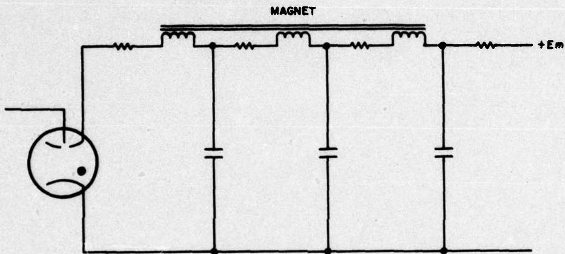
Figure 11. Alternate field shaping circuit.
