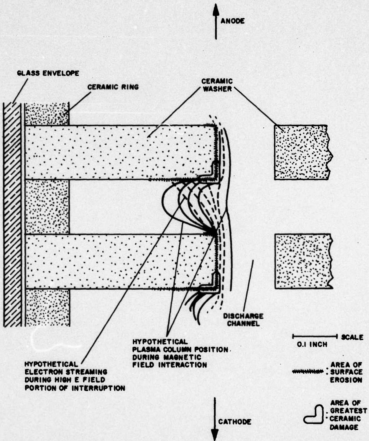
Figure 6. RSI 005 during magnetic field interaction.
