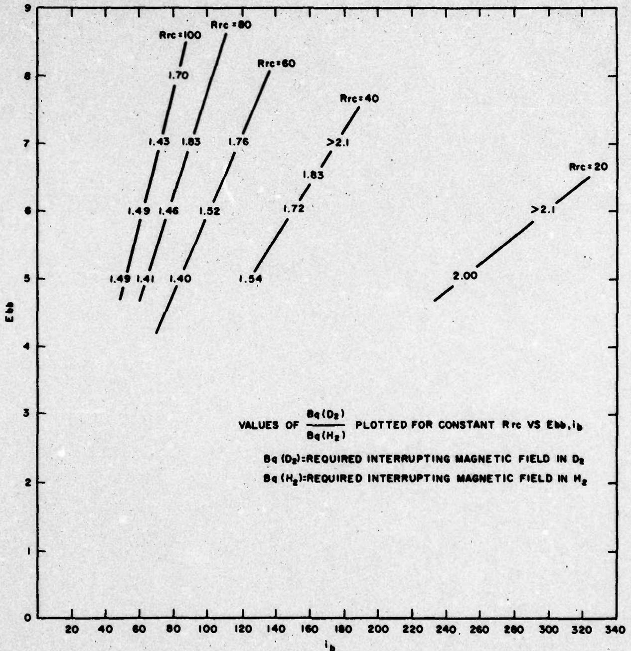
Figure 5. Interrupting magnetic field in deuterium vs. hydrogen as a function of Ebb,  $I_b$  for RSI 004.
