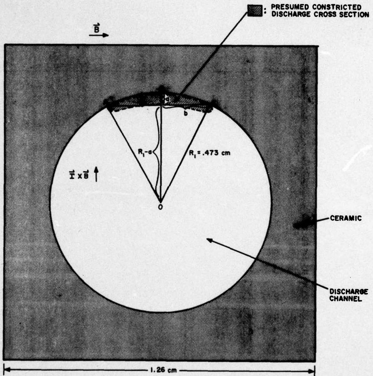
Figure 16. RSI 003 tube and discharge cross-section dimensions.
