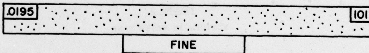
FIGURE 4 - POROSITY REFERENCE CHART.
