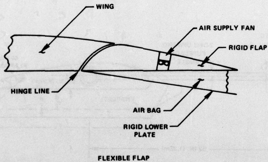
Figure 3 - Model Flap Configurations
