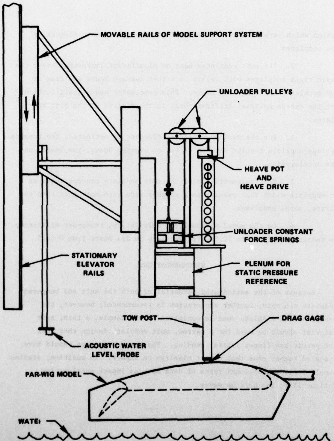
Figure 1 - PAR-WIG Model on Carriage III Support System
