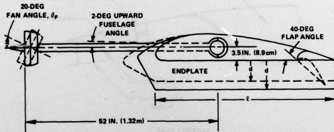
Figure 2 - General Arrangement of PAR-WIG Model
