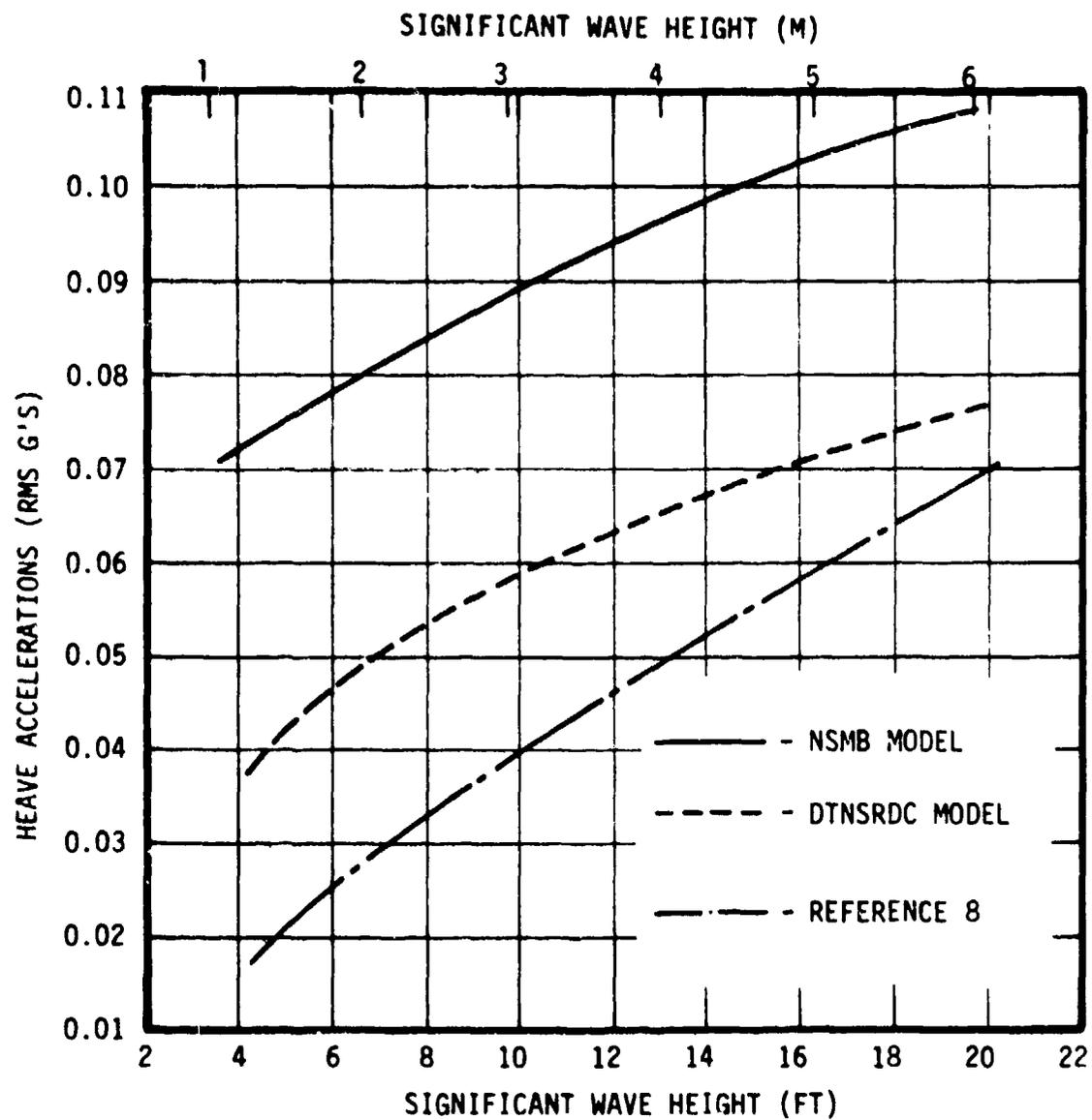
Figure 17 - Heave Accelerations of 640,000 Pound (291,000 Kilogram)
