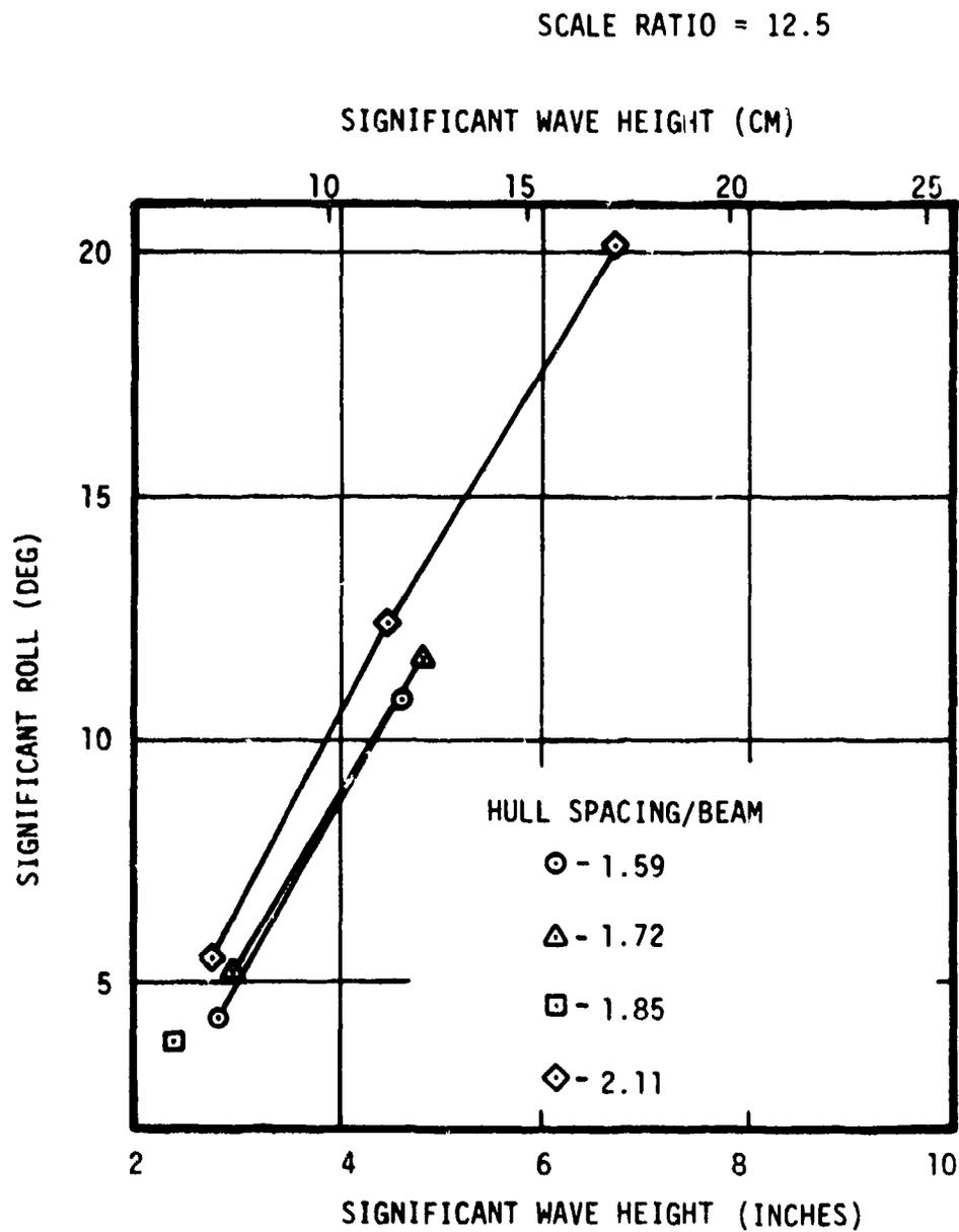
Figure 13 - Roll Displacements of DTNSRDC Model in Beam Seas
