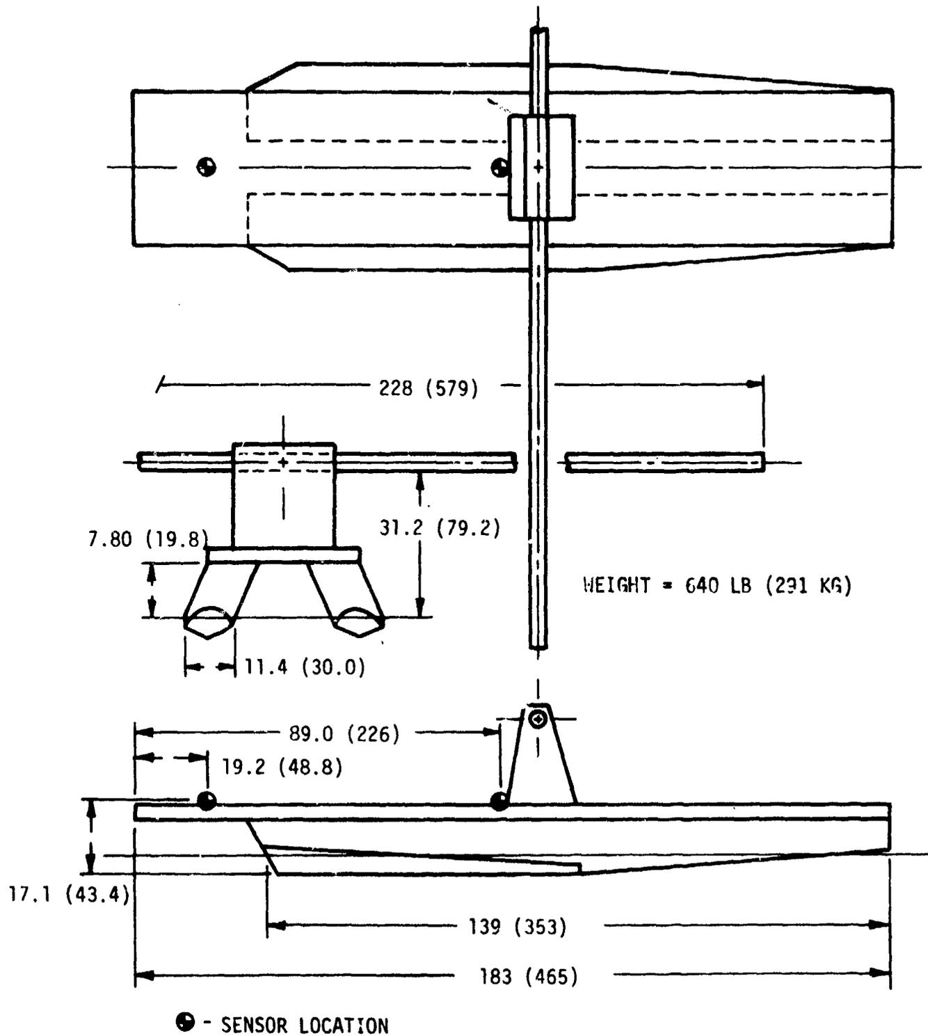
Figure 7 - General Arrangement of DTNSRDC Model 1
