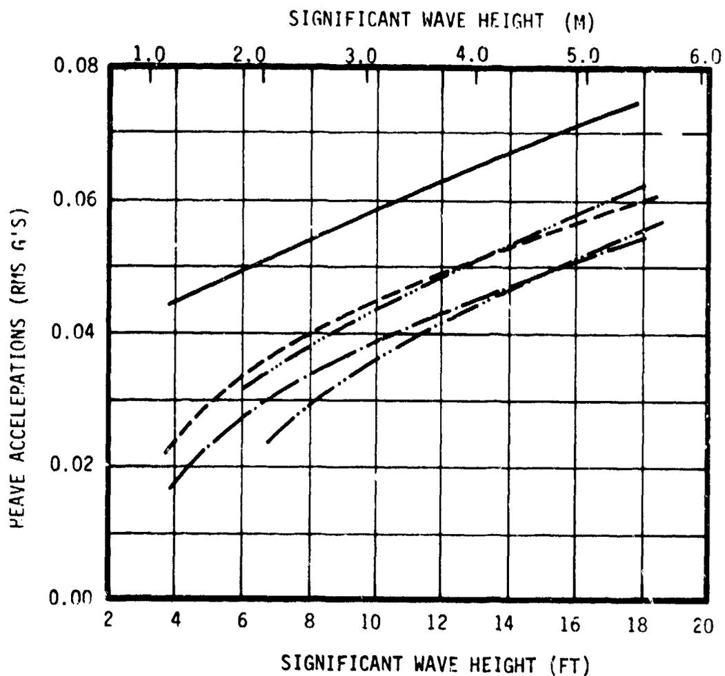
Figure 15 - Heave Accelerations of 1,250,000 Pound (568,000 Kilogram) Aircraft in Head Seas
