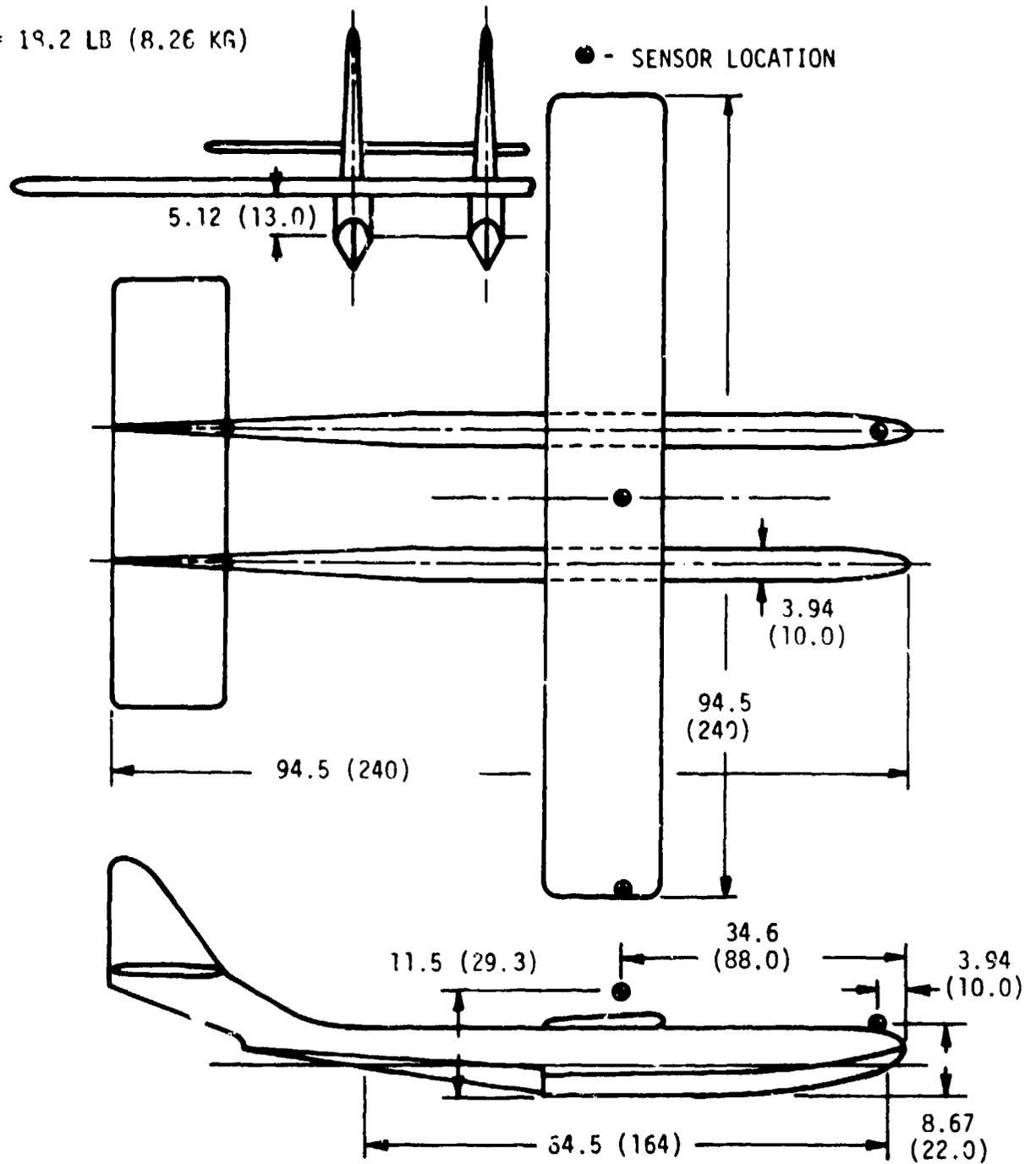
Figure 3 - General Arrangement of NSMB Model
