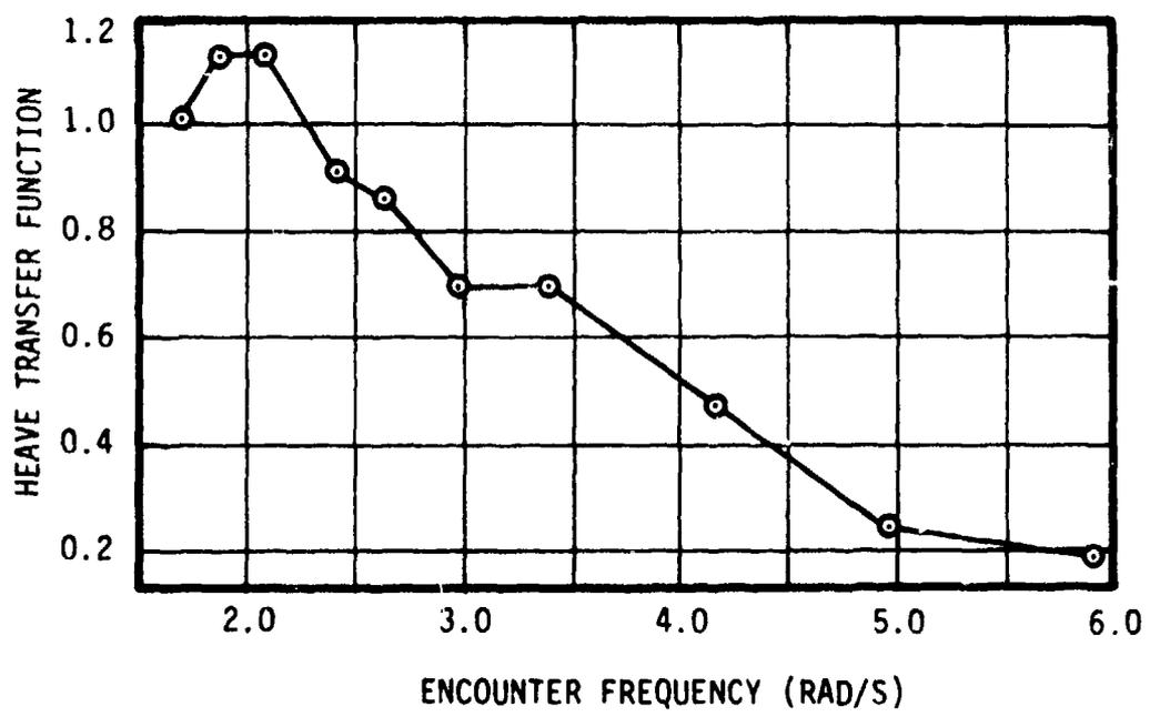
Figure 9 - Transfer Functions of DTNSRDC Model in Head Seas
