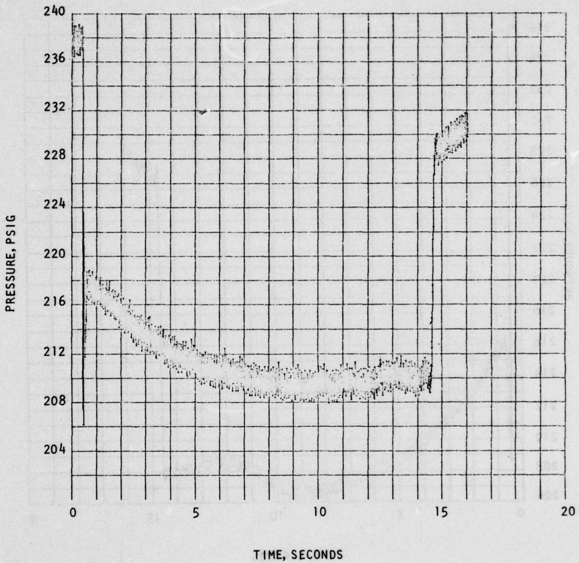
Figure 92. TEM-2 First Burn (Test 846-013) NTO Inlet Pressure
