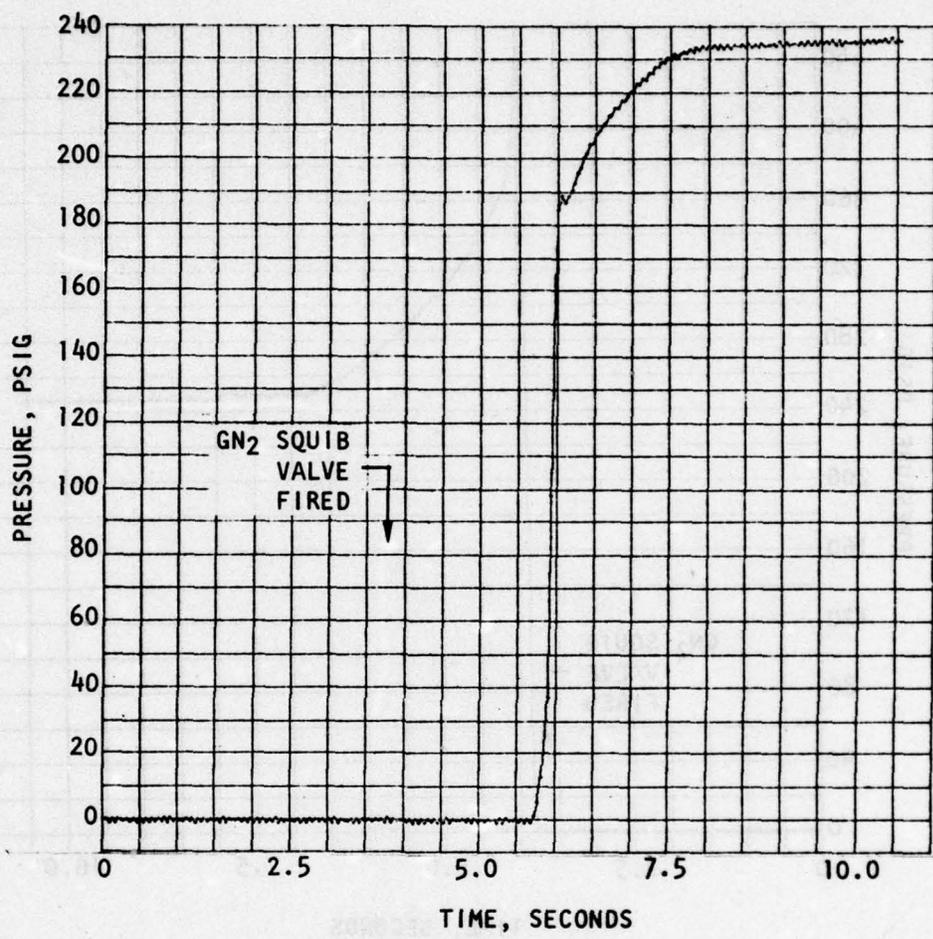
Figure 80. TEM-1 Pressurization Transient MMH Inlet Pressure
