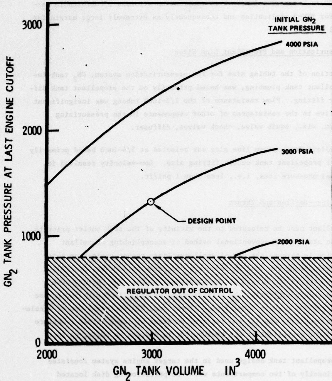
Figure 1. TES Pressurization Requirements
