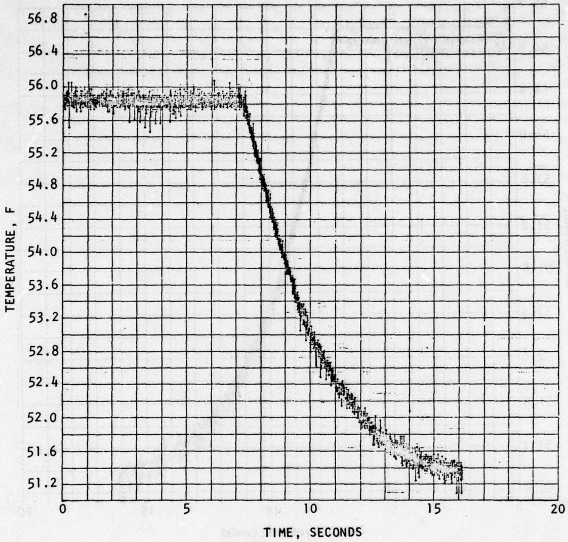
Figure 110. TEM-3 First Burn (Test 846-001) NTO Temperature
