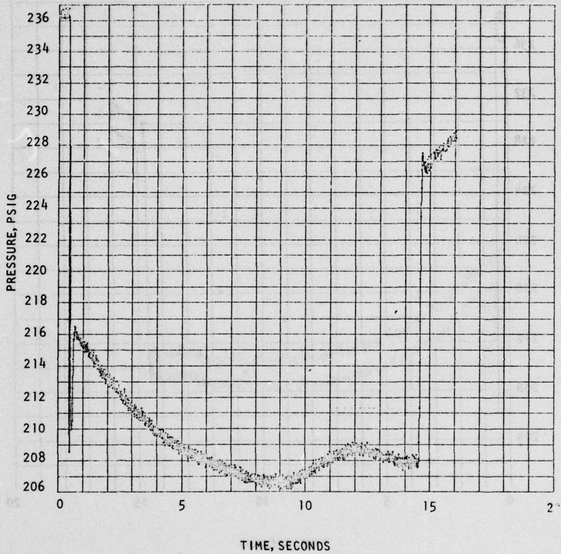
Figure 91. TEM-2 First Burn (Test 846-013) MMH Inlet Pressure
