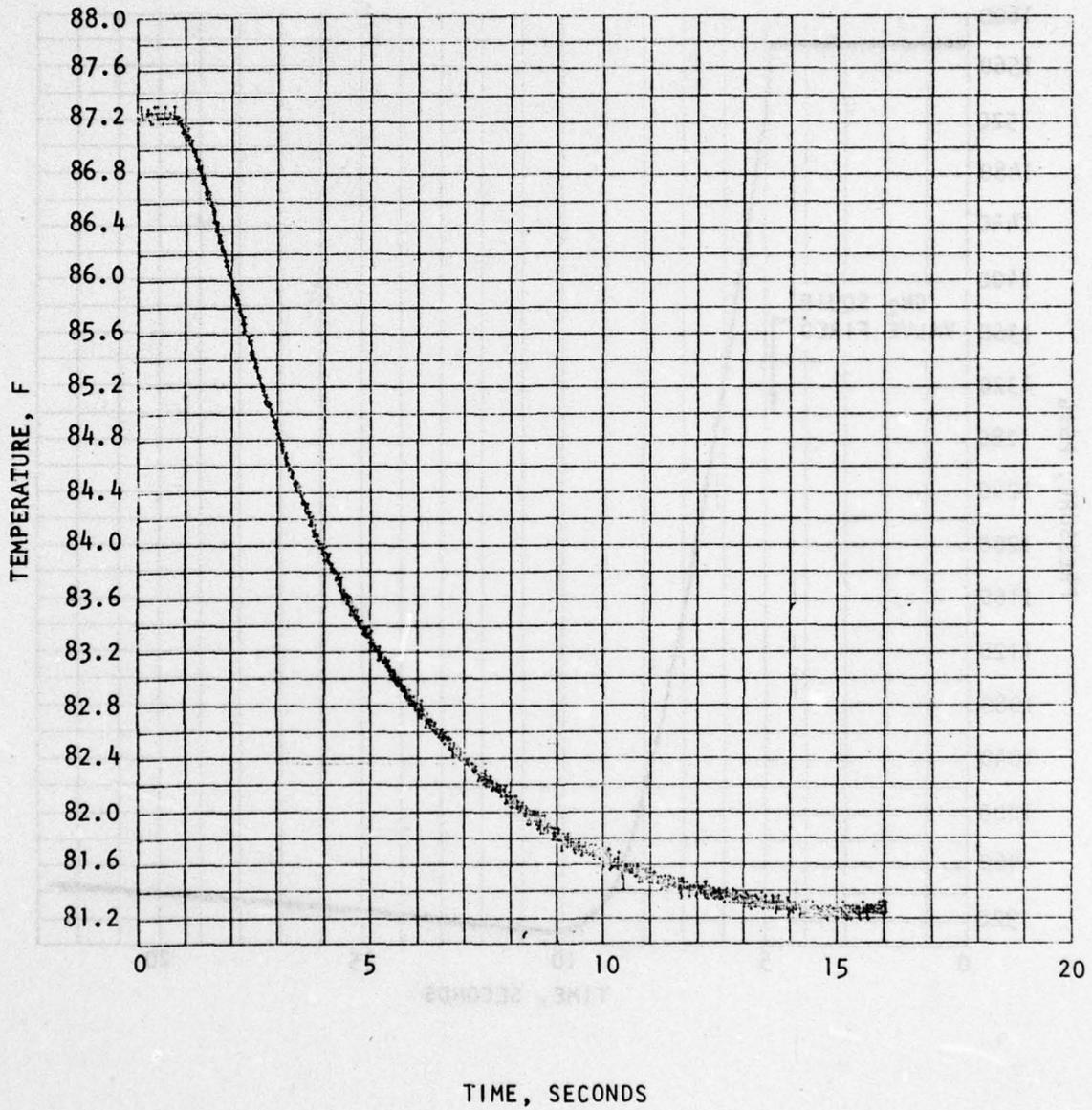
Figure 97. TEM-2 First Burn (Test 846-013) NTO Temperature
