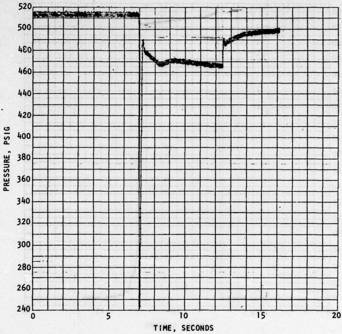
Figure 104. TEM-3 First Burn (Test 846-001) MMH Inlet Pressure
