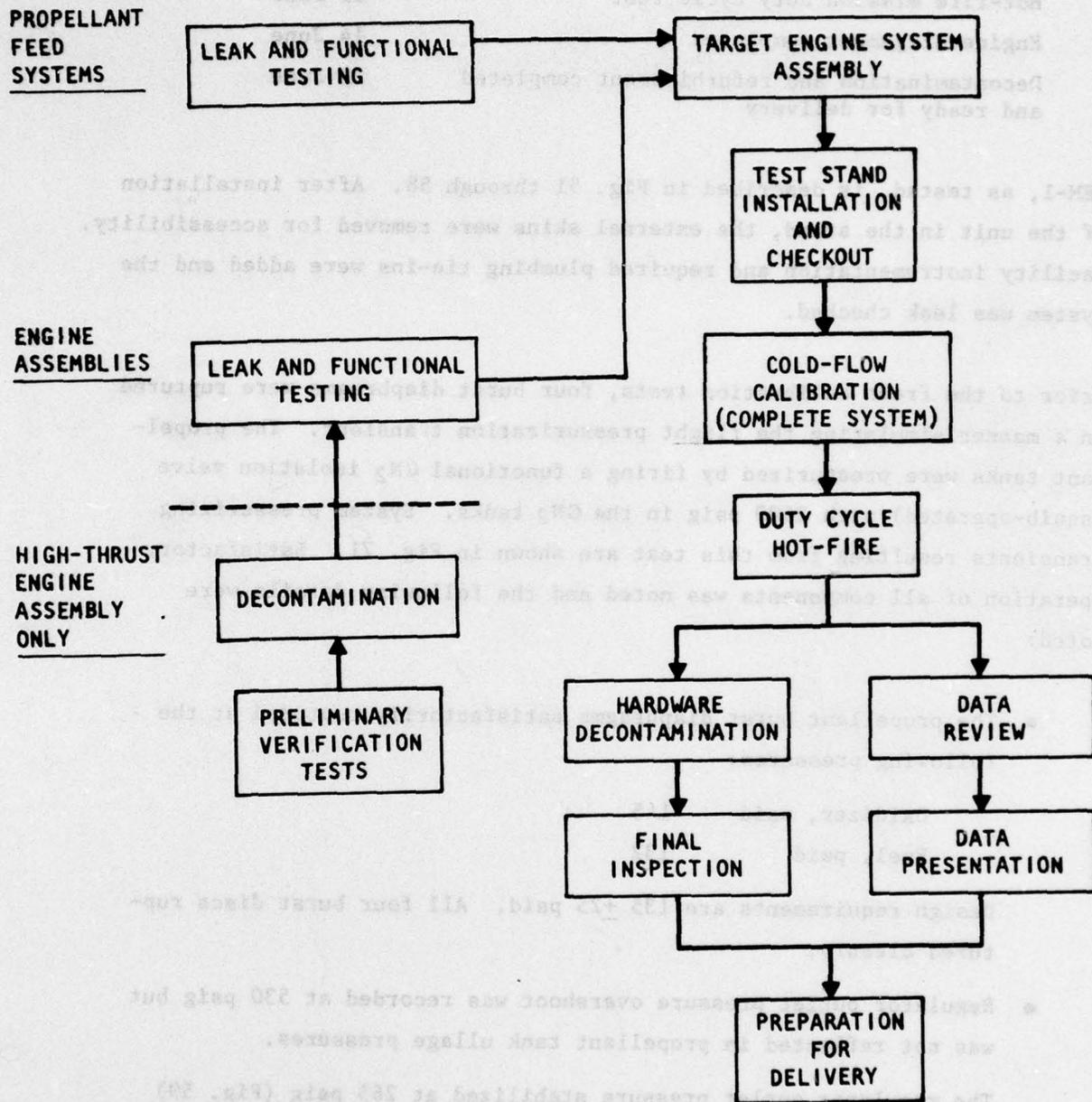
Figure 50. TES Functional Verification Process Flow
