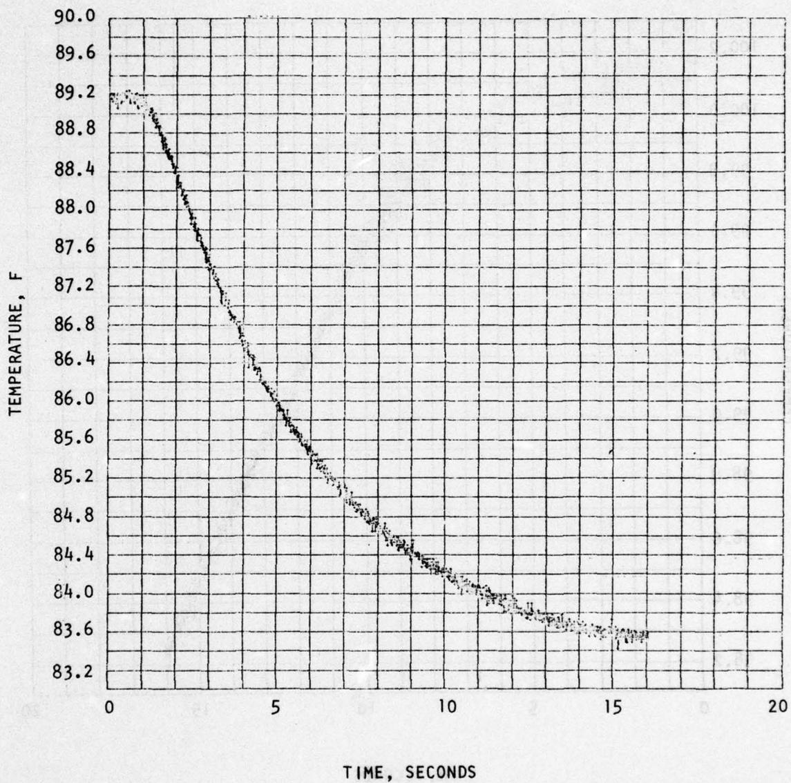
Figure 96. TEM-2 First Burn (Test 846-013) MMH Temperature
