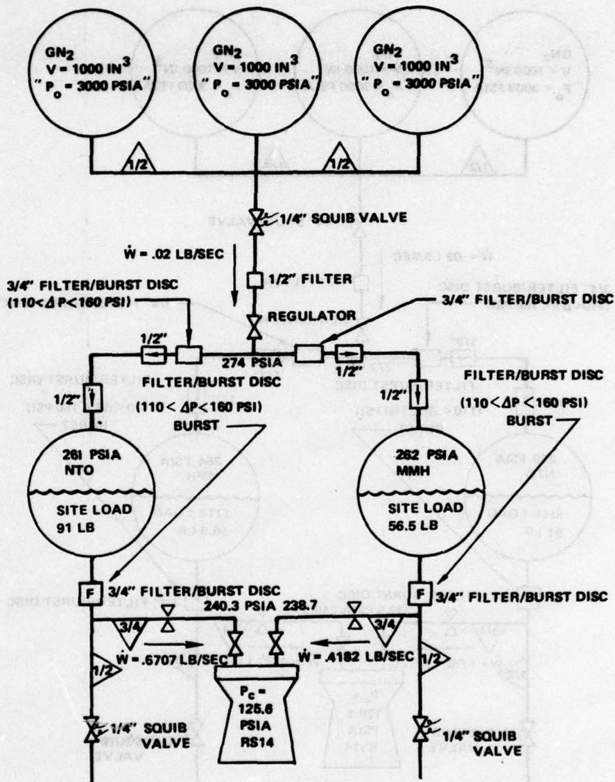
Figure 7. TEM-2 Pressure/Flow Schedule (Test Results)
