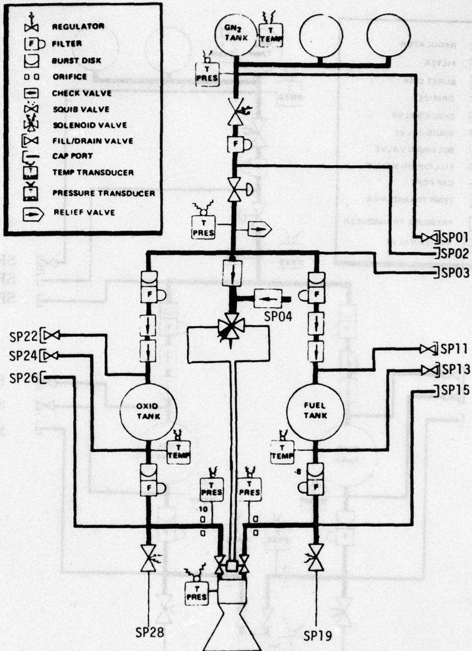
Figure 49. TES TEM-3 Schematic
