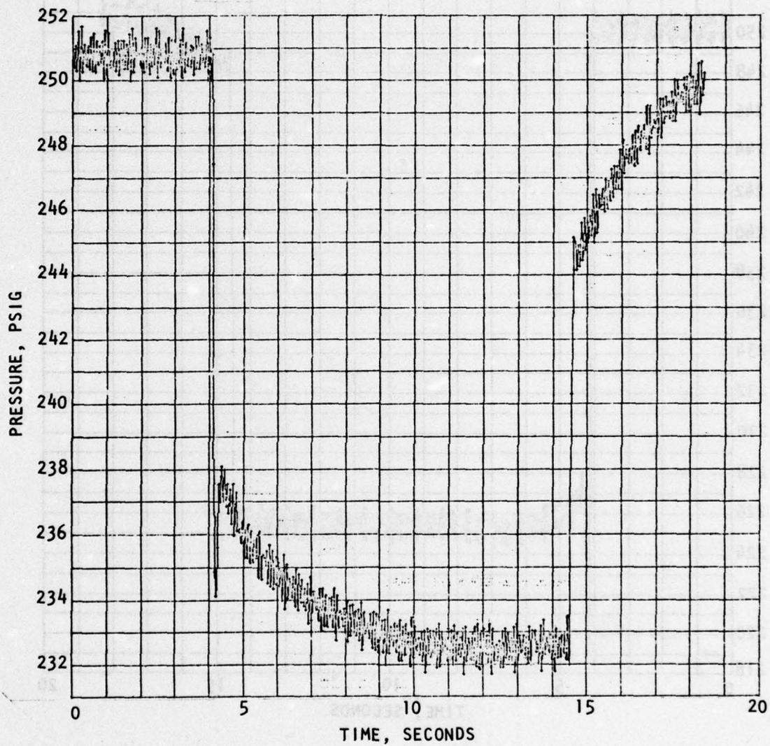
Figure 83. TEM-1 First Burn (Test 846-006) MMH Inlet Pressure
