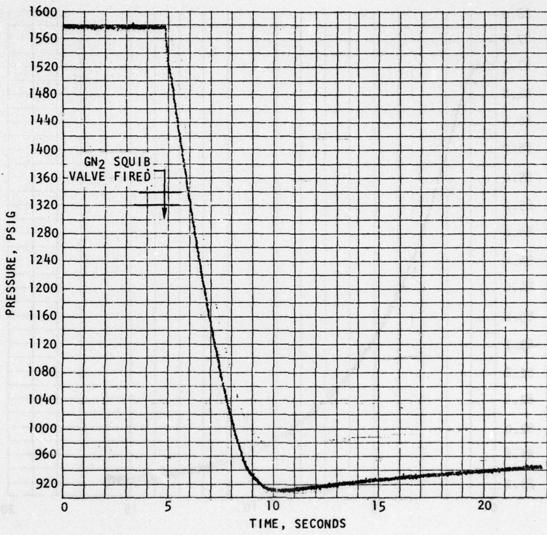
Figure 98. TEM-3 Pressurization Transient GN<sub>2</sub> Tank Pressure
