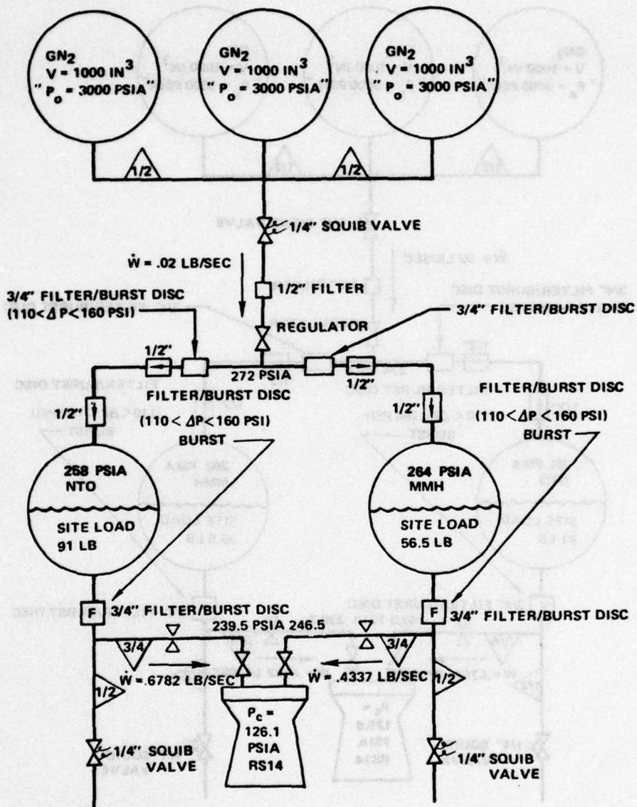
Figure 6. TEM-1 Pressure/Flow Schedule (Test Results)
