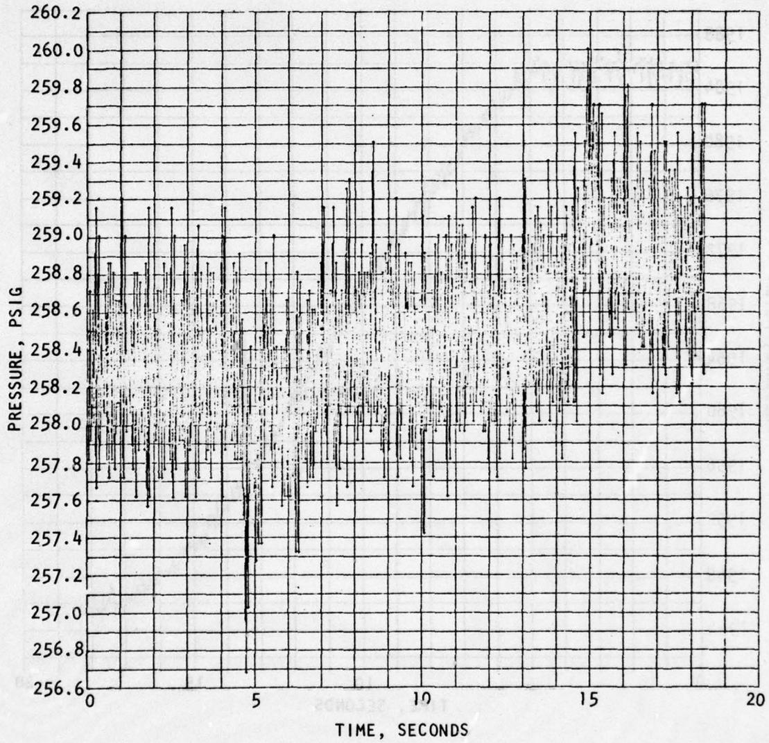
Figure 85. TEM-1 First Burn (Test 846-006) Regulator Outlet Pressure
