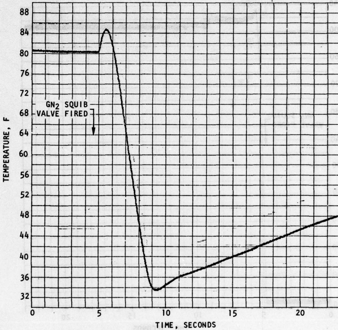
Figure 99. TEM-3 Pressurization Transient GN<sub>2</sub> Tank Temperature
