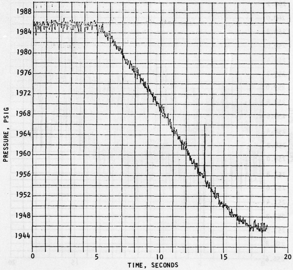
Figure 86. TEM-1 First Burn (Test 846-006) GN<sub>2</sub> Tank Pressure
