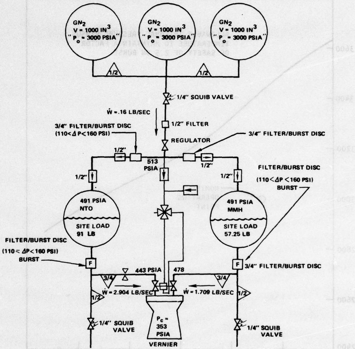
Figure 8. TEM-3 Pressure/Flow Schedule (Test Results)
