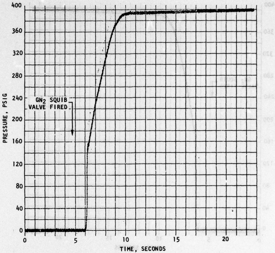
Figure 101. TEM-3 Pressurization Transient MMH Inlet Pressure
