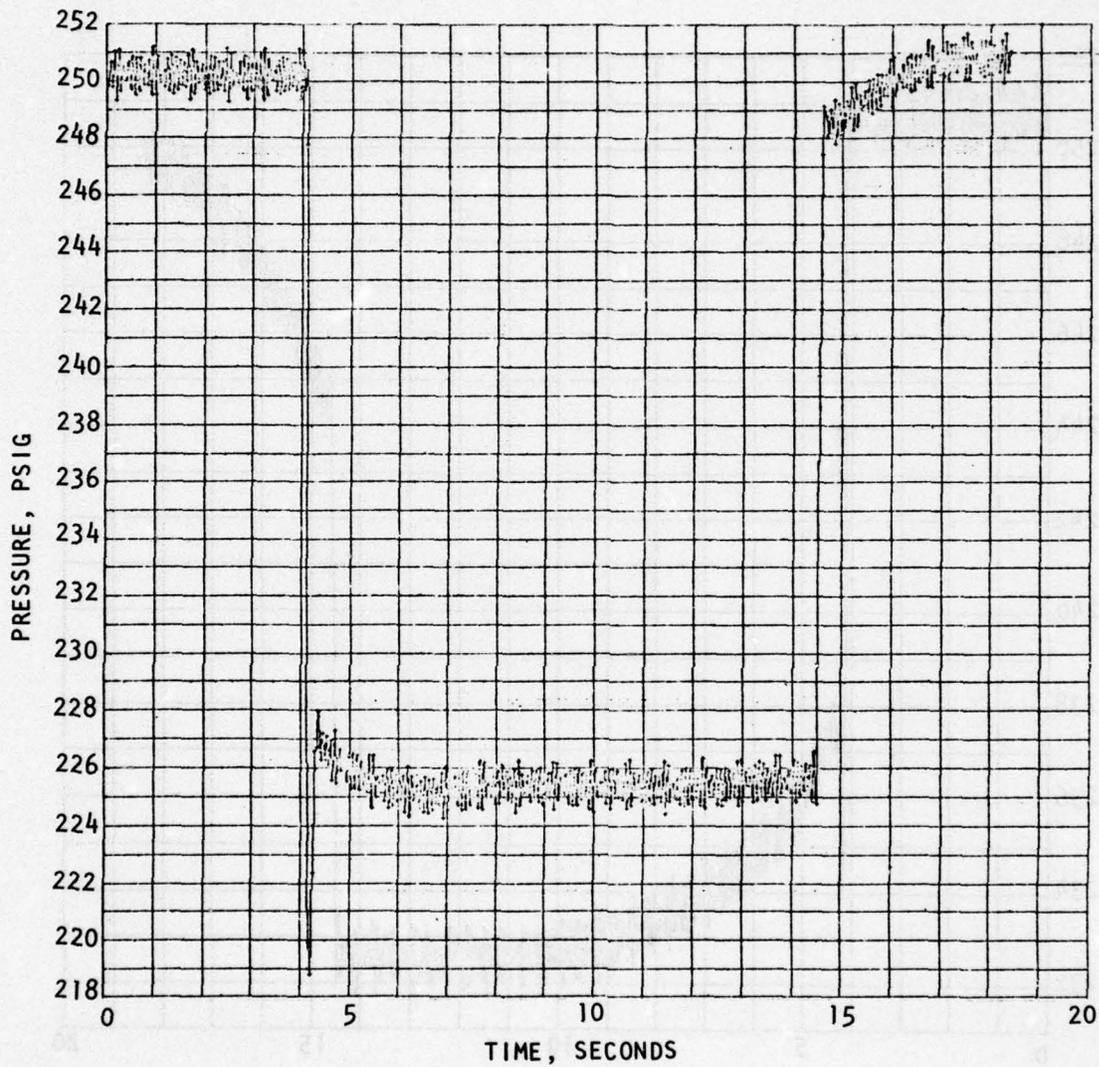
Figure 84. TEM-1 First Burn (Test 846-006) NTO Inlet Pressure
