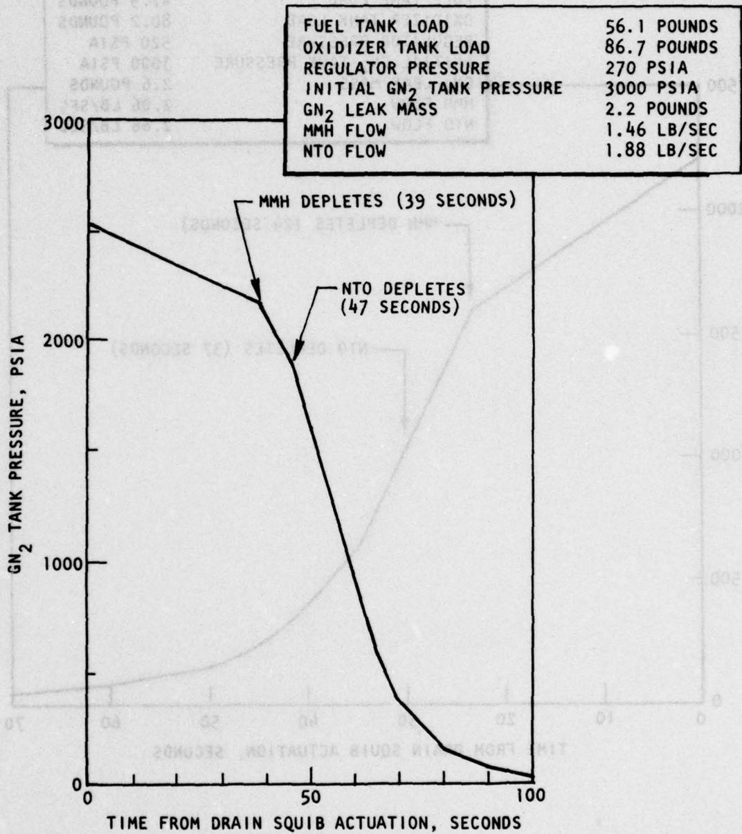
Figure 11. TEM-1 Propellant Dump (Model Simulation)
