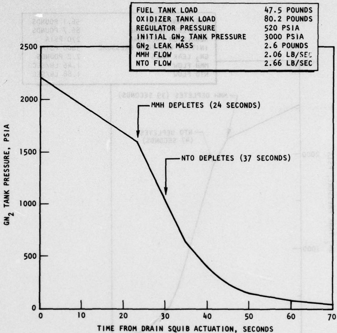
Figure 12. TEM-3 Propellant Dump (Model Simulation)
