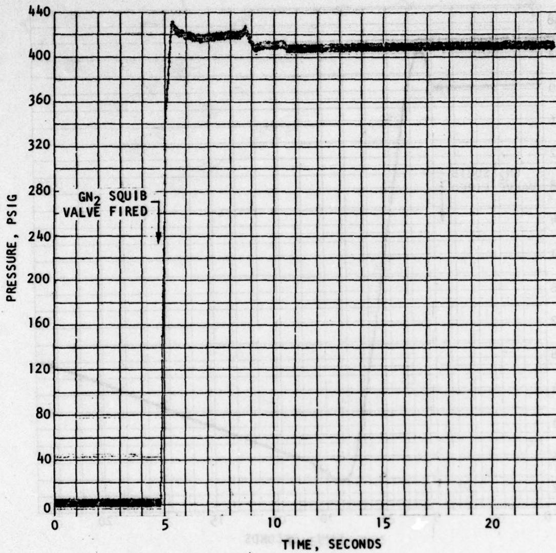
Figure 100. TEM-3 Pressurization Transient Regulator Outlet Pressure
