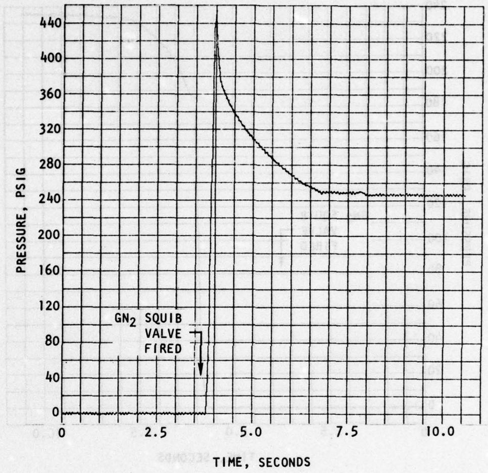
Figure 79. TEM-1 Pressurization Transient Regulator Outlet Pressure
