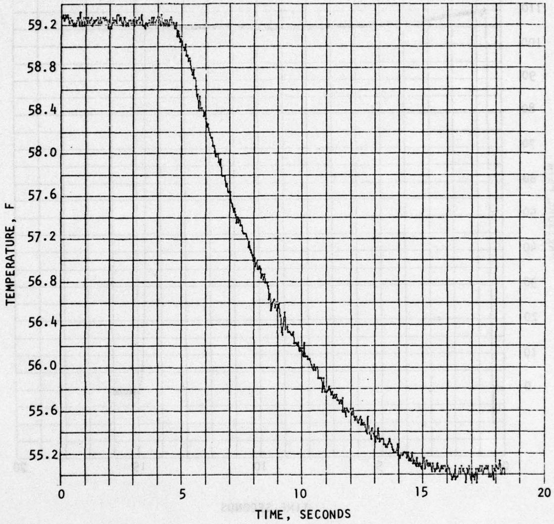
Figure 89. TEM-1 First Burn (Test 846-006) NTO Temperature
