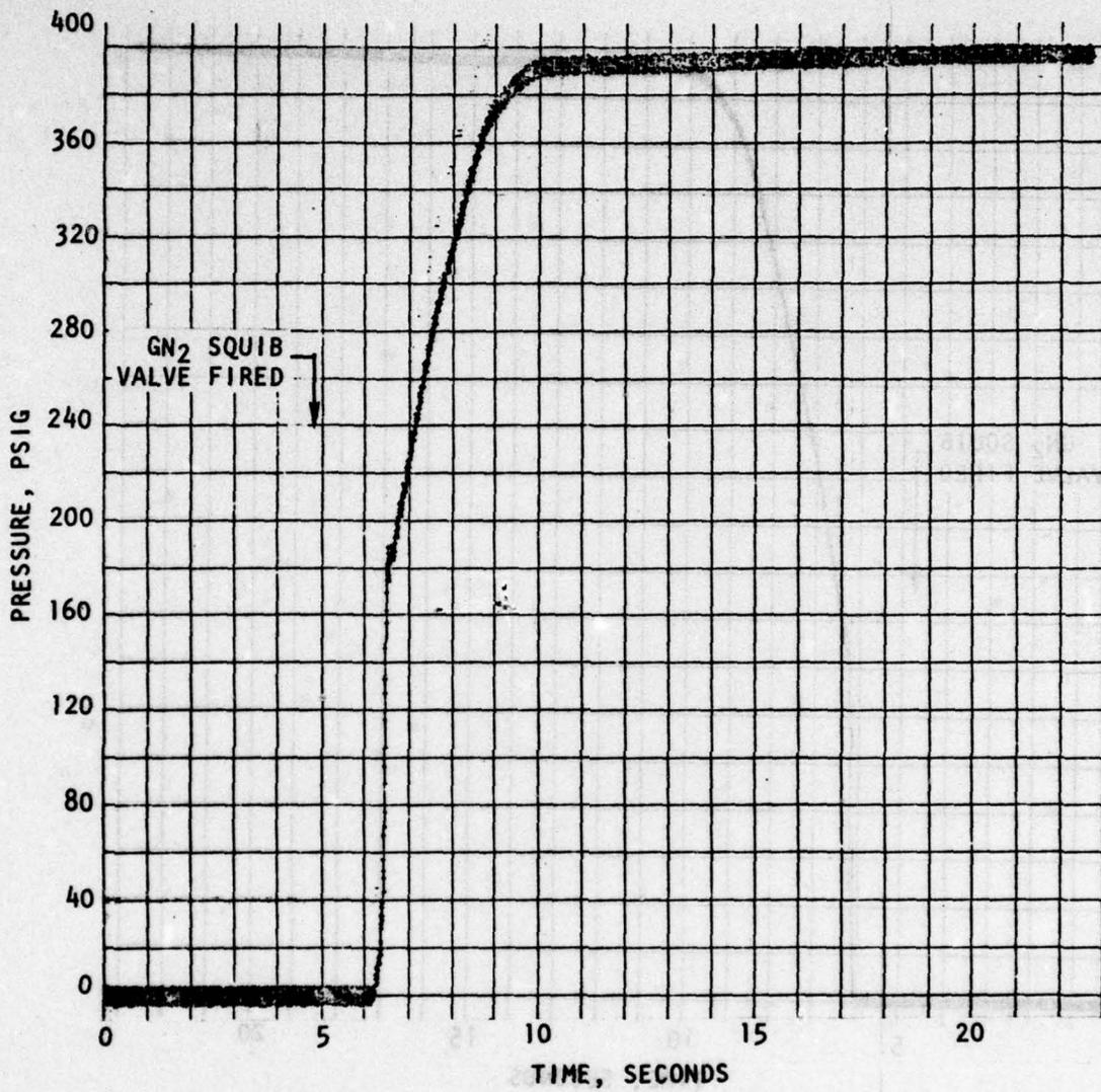
Figure 102. TEM-3 Pressurization Transient NTO Inlet Pressure
