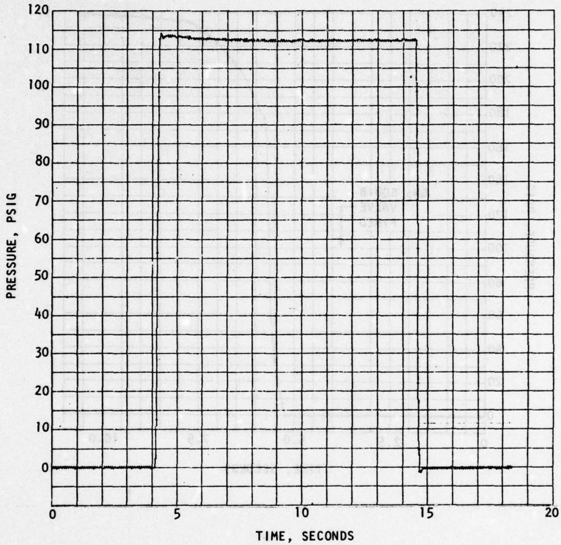
Figure 82. TEM-1 First Burn (Test 846-006) Chamber Pressure
