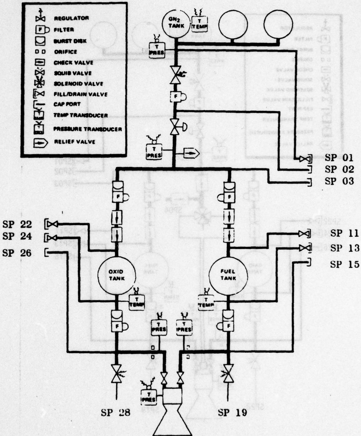
Figure B-1. TEM-1 and -2 Schematic
