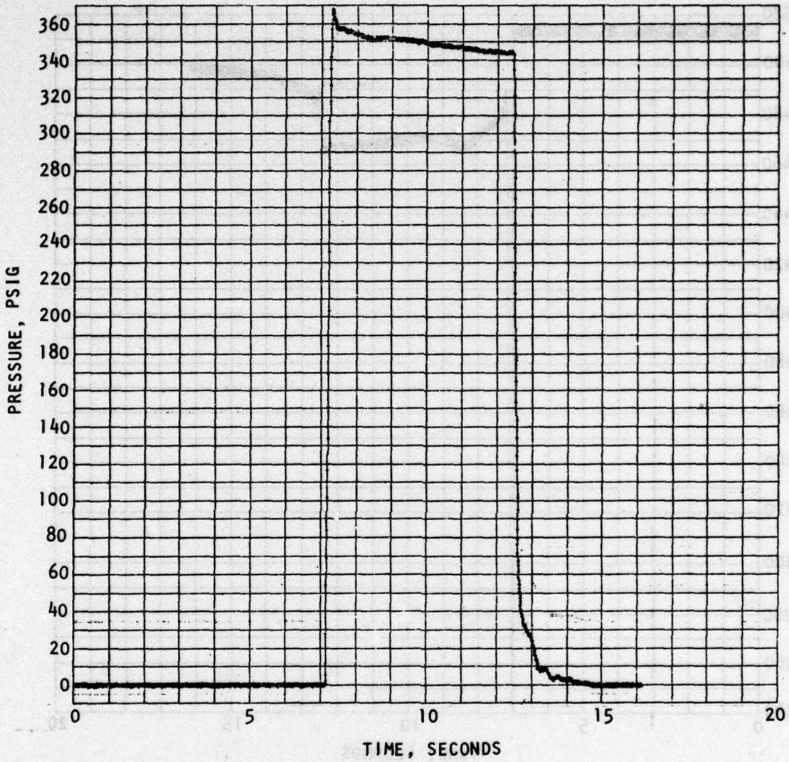
Figure 103. TEM-3 First Burn (Test 846-001) Chamber Pressure
