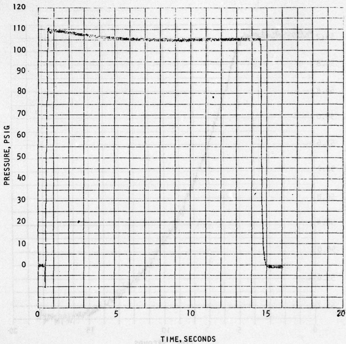
Figure 90. TEM-2 First Burn (Test 846-013) Chamber Pressure
