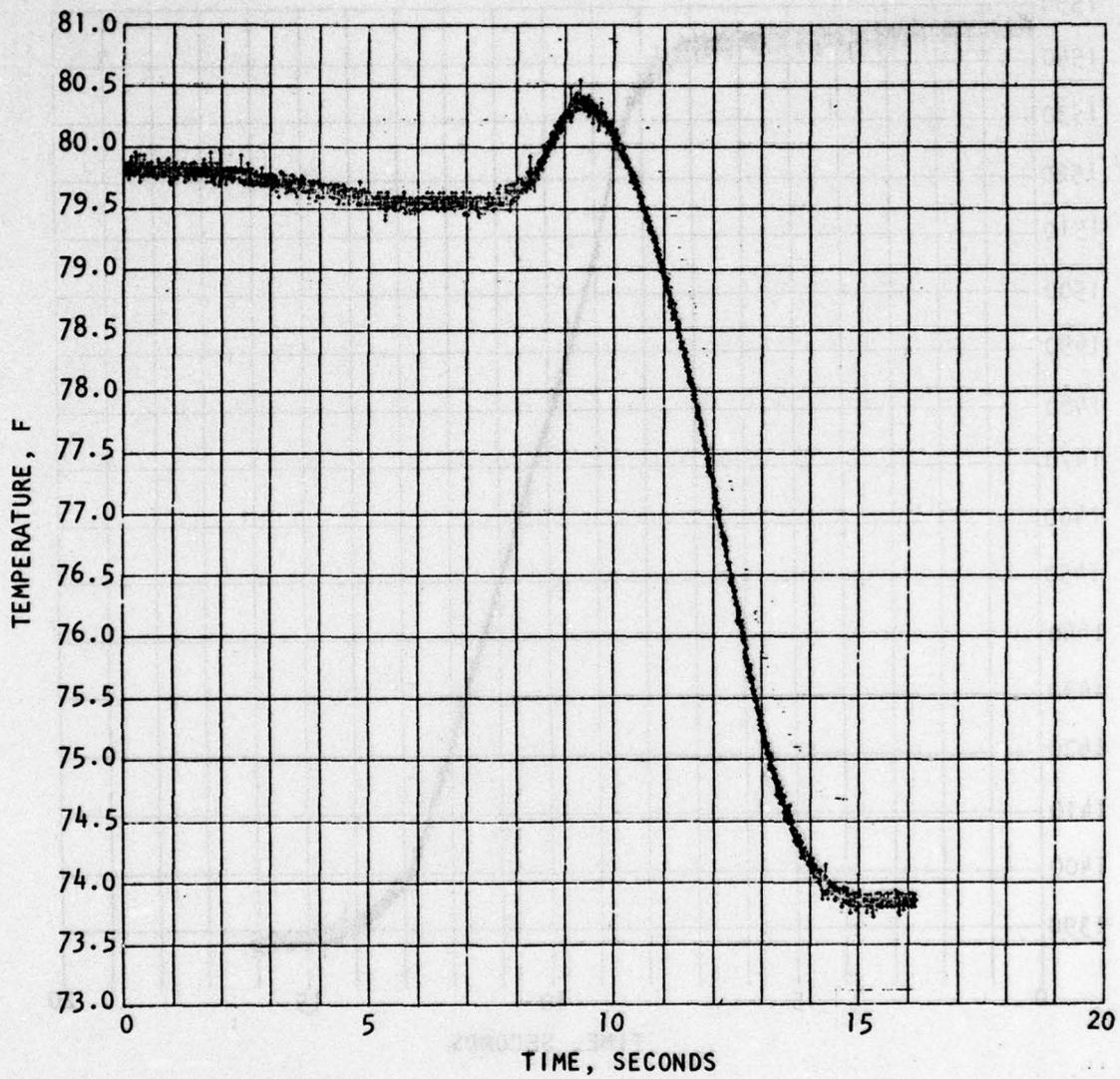
Figure 108. TEM-3 First Burn (Test 846-001) GN<sub>2</sub> Tank Temperature
