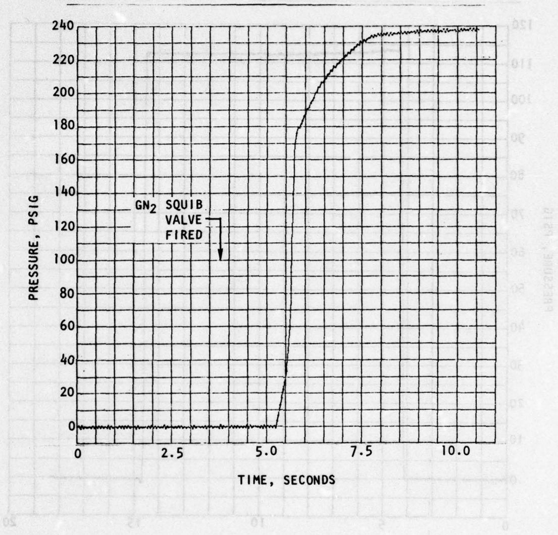
Figure 81. TEM-1 Pressurization Transient NTO Inlet Pressure
