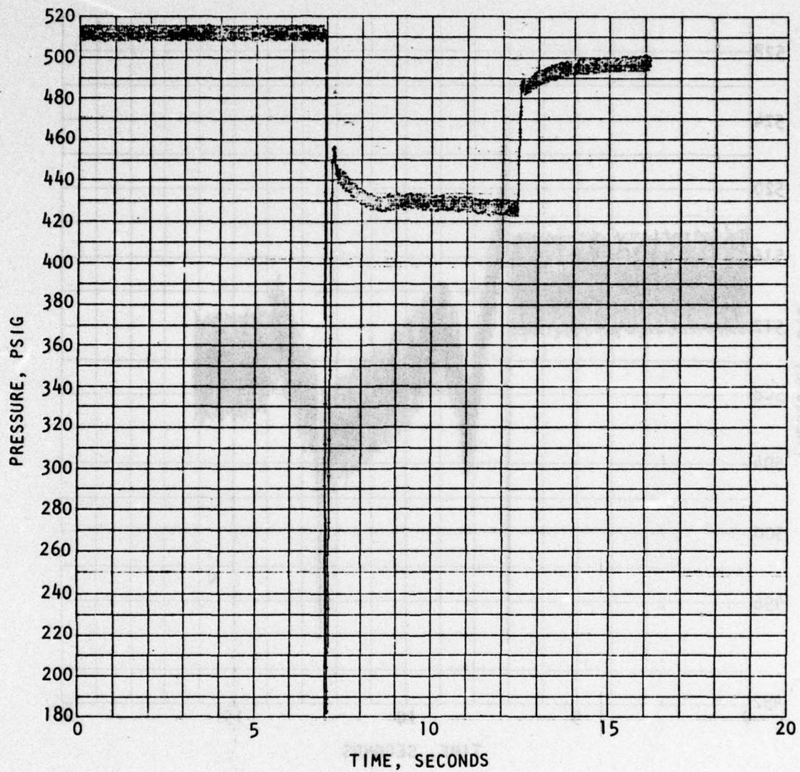
Figure 105. TEM-3 First Burn (Test 846-001) NTO Inlet Pressure
