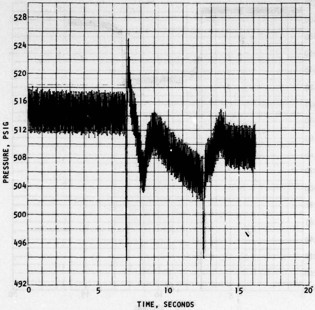
Figure 106. TEM-3 First Burn (Test 846-001) Regulator Outlet Pressure
