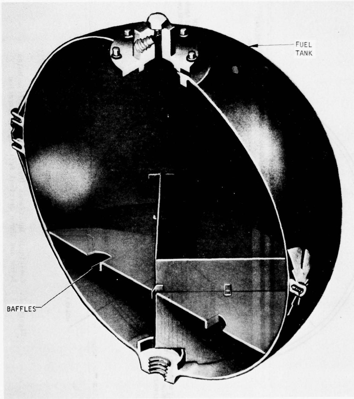
Figure 3. TES Propellant Tank
