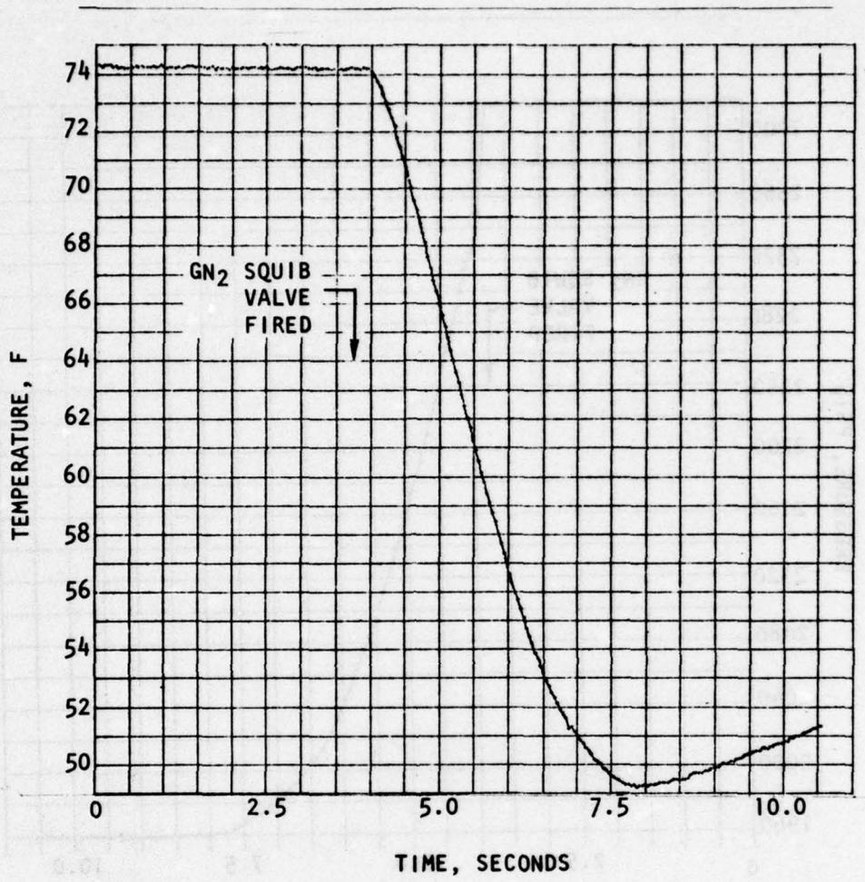
Figure 78. TEM-1 Pressurization Transient GN<sub>2</sub> Tank Temperature
