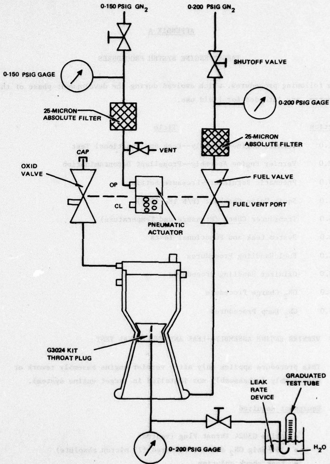
Figure A-1. Vernier Engine Assembly Functional Test
