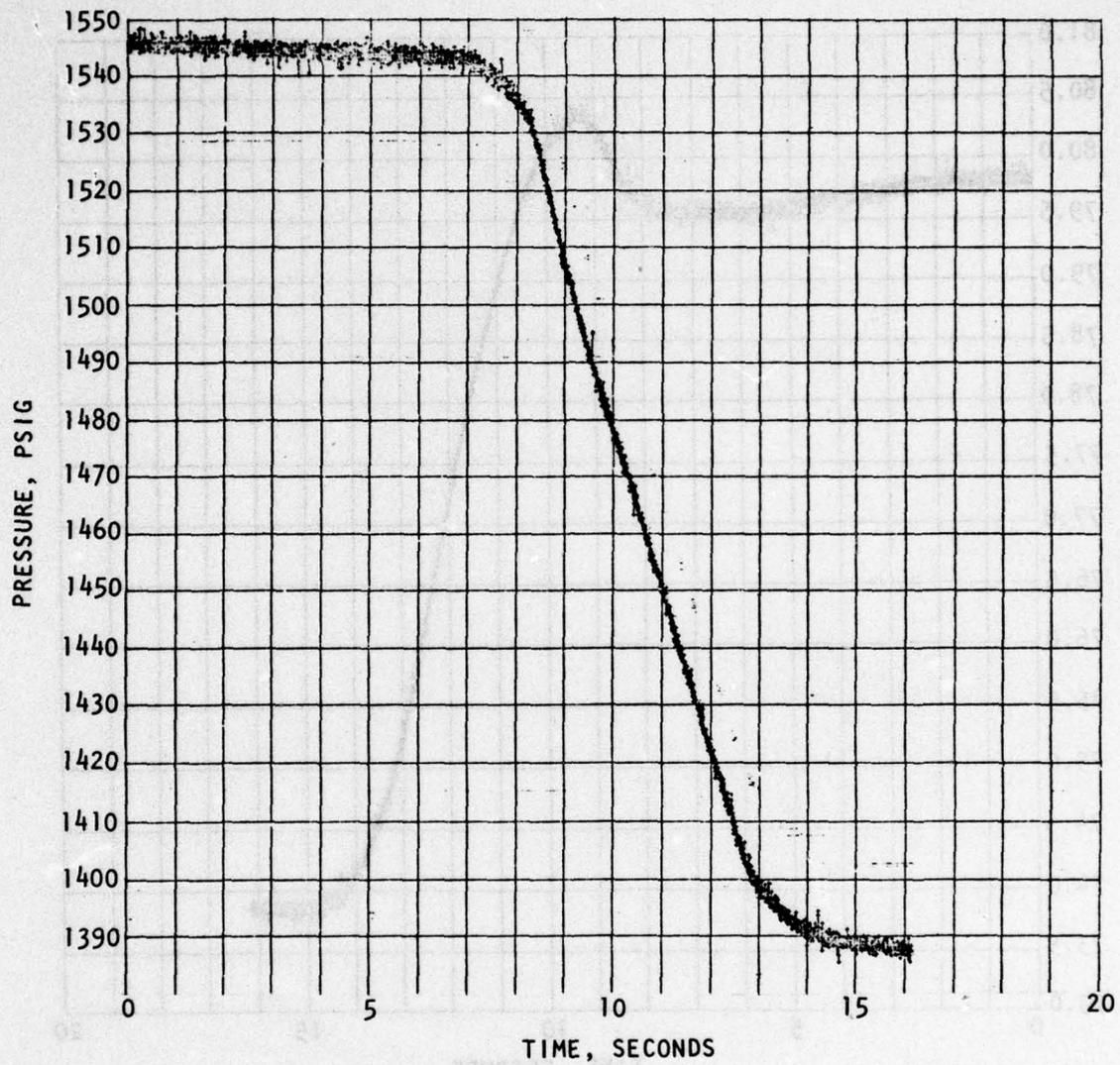
Figure 107. TEM-3 First Burn (Test 846-001) GN<sub>2</sub> Tank Pressure
