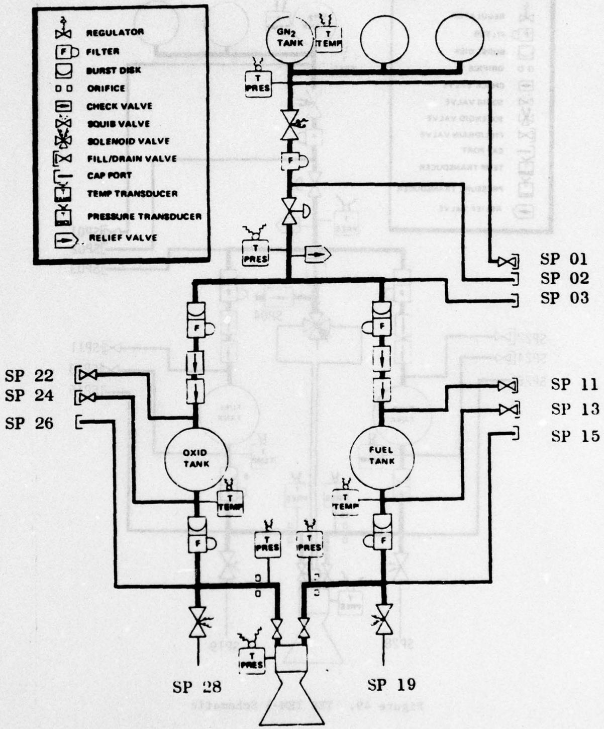
Figure 48. TES TEM-1 and -2 Schematic
