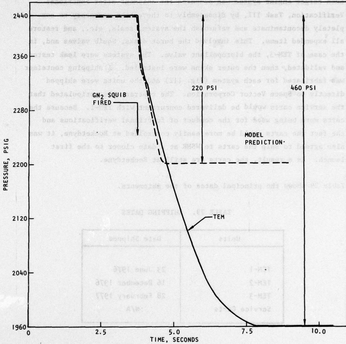
Figure 111. TEM-1 Pressurization Transient GN<sub>2</sub> Tank Pressure
