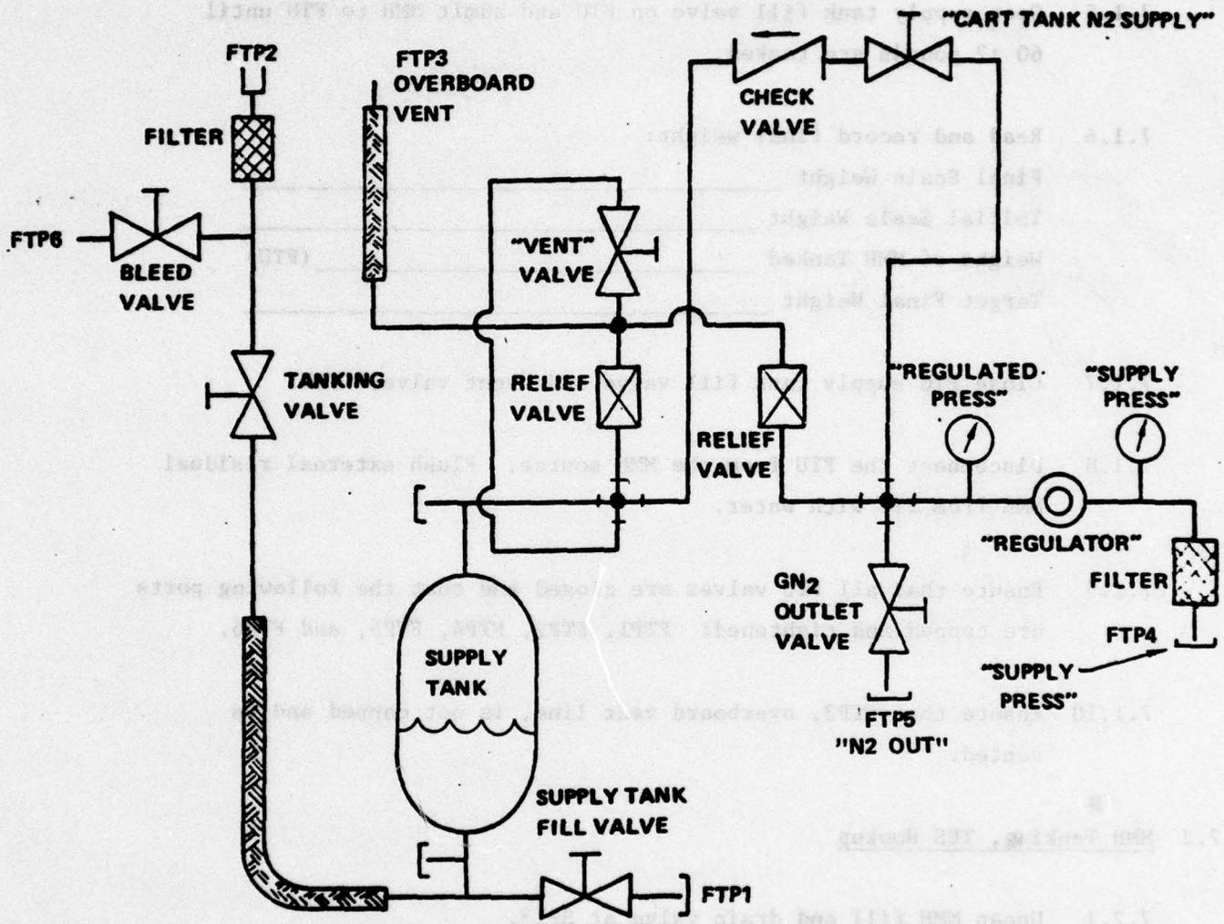
Figure A-6. Fuel Tanking Unit (FTU)
