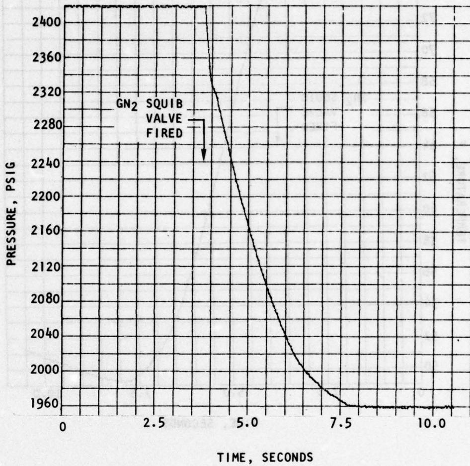
Figure 77. TEM-1 Pressurization Transient GN<sub>2</sub> Tank Pressure
