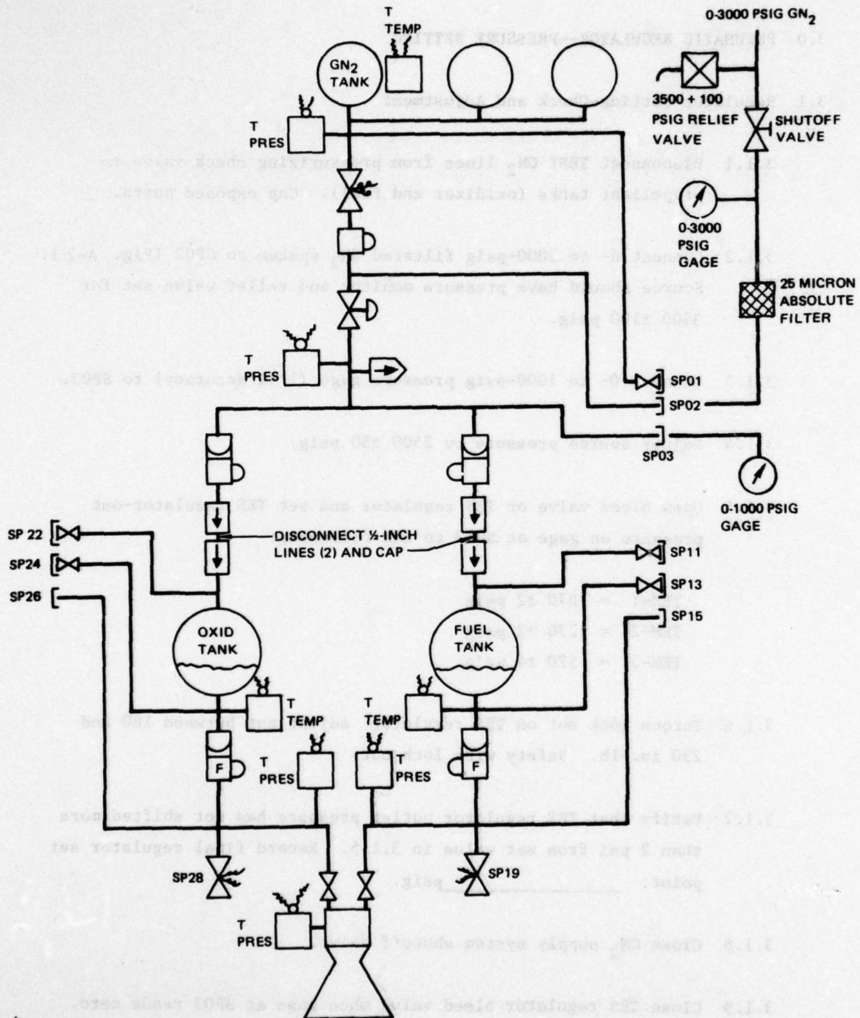
Figure A-2. Pneumatic Regulator - Pressure Setting
