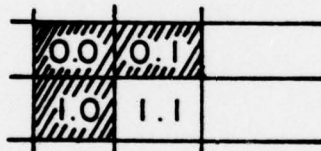
Fig. 43: The one step predictor. The Fig. shows the pixels that take part in the one-step-predictor of pixel 1,1
