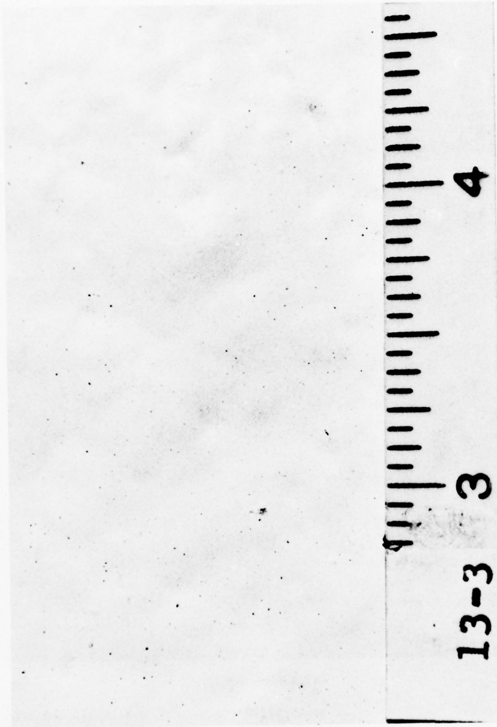
Figure 15. Excellent clean and glossy surface of catalyzed urethane (System 13) after 1 year at China Lake.
