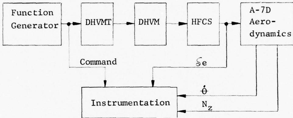
FIGURE 87 Phase III DAIS Test Set-Up
