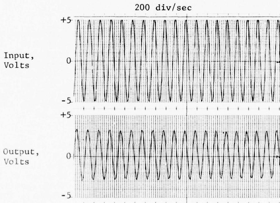
FIGURE 74 40 Hz Input-Output at
