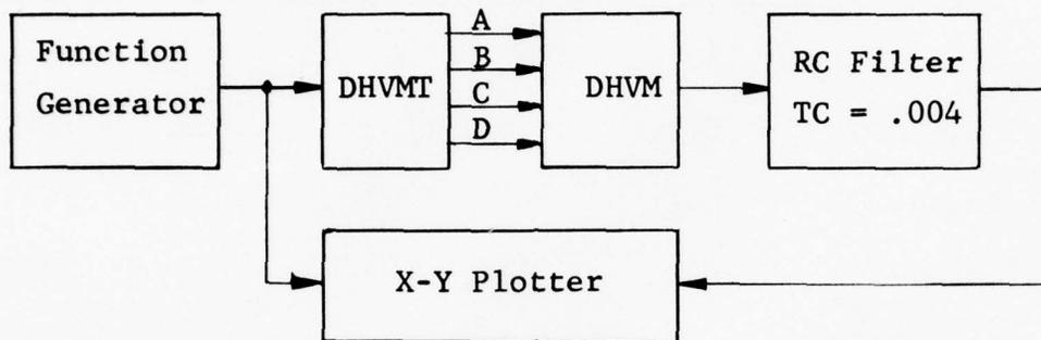
FIGURE 11 Resolution and Linearity Test Set-Up
