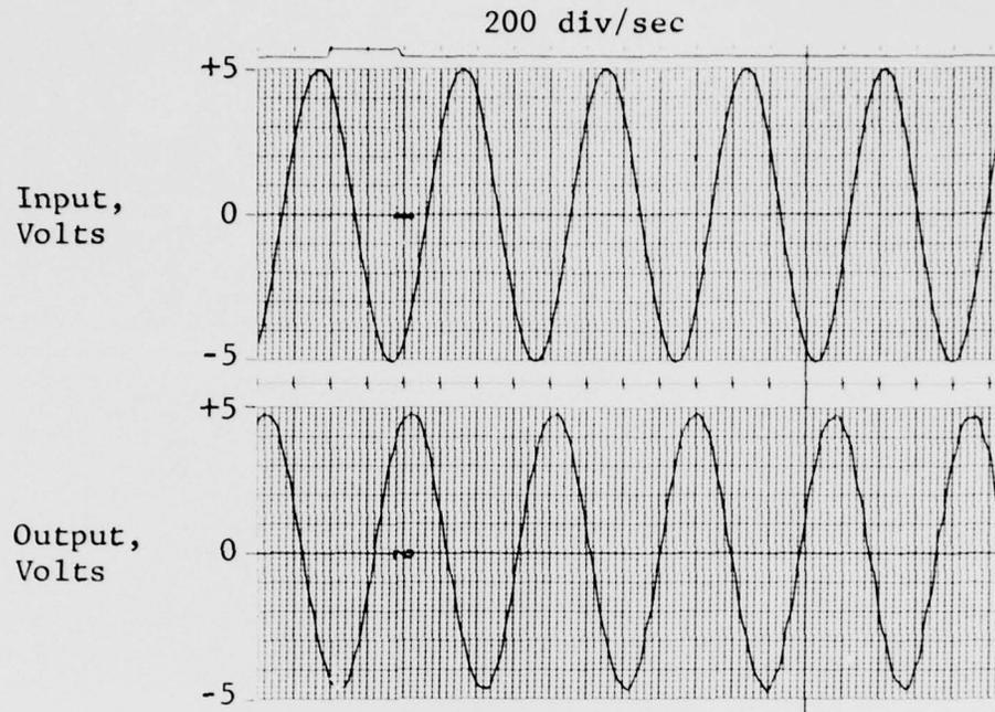
FIGURE 52 10 Hz Input-Output at 125 samples/sec.
