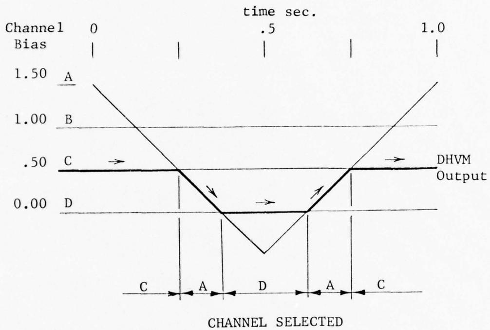
FIGURE 23 Low Median Signal Selection
