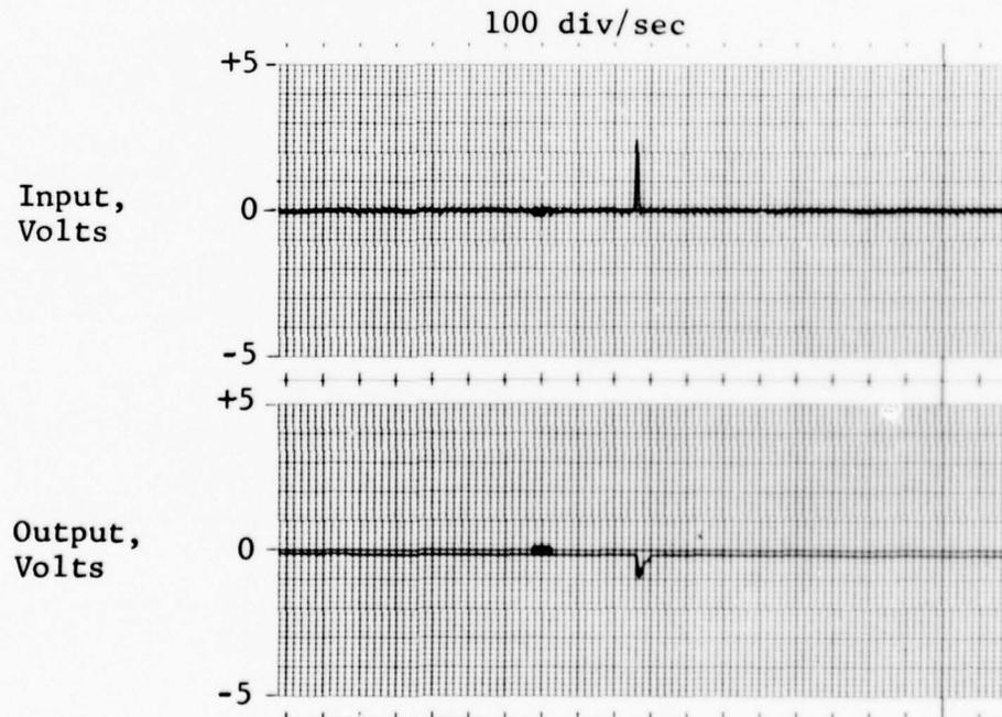
FIGURE 78 Third Failure Transients with 5 Errors
