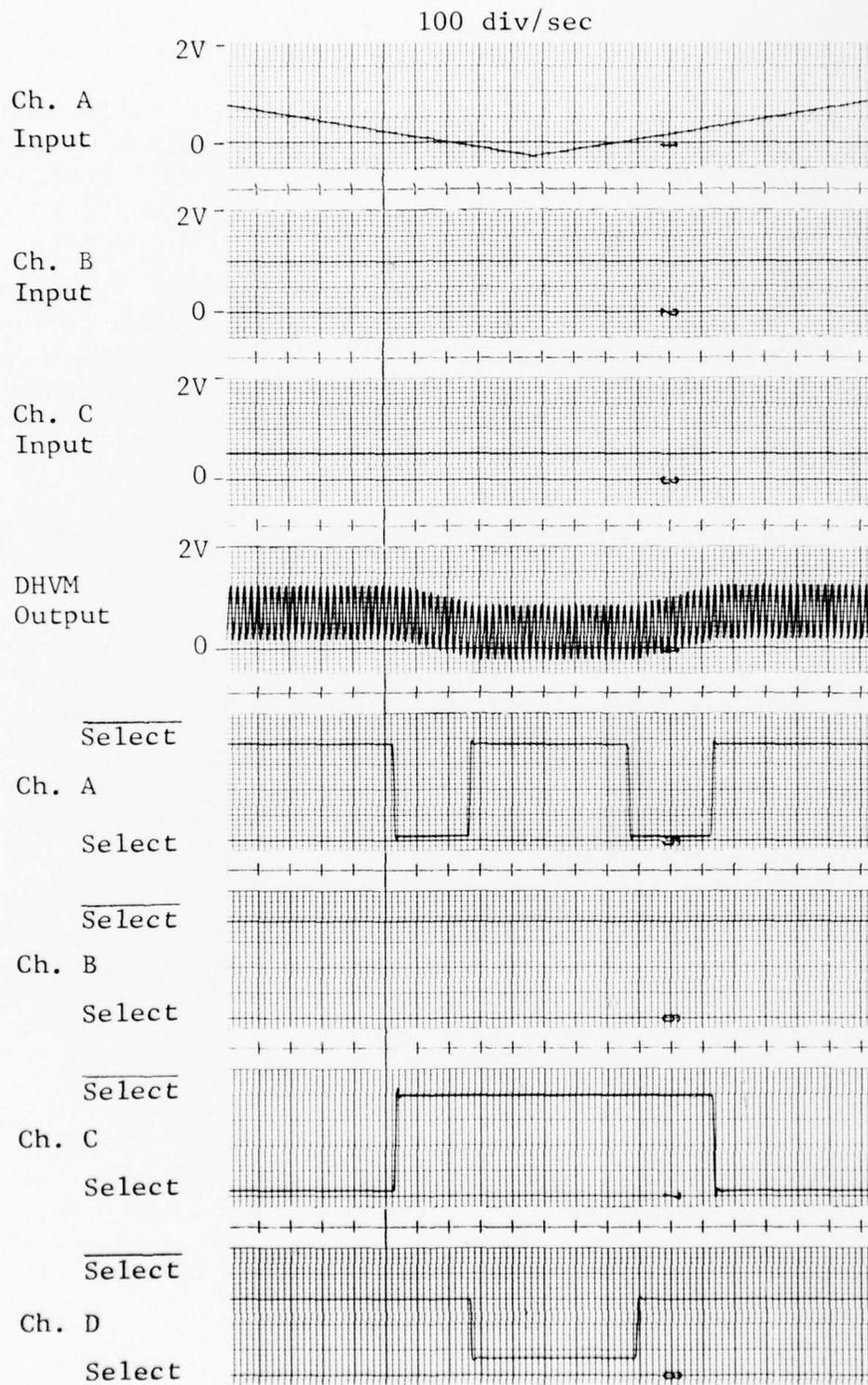
FIGURE 25 Channel Select Delay
