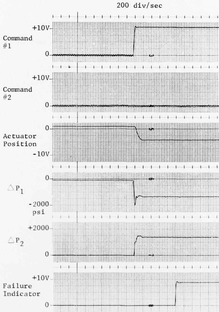
FIGURE 101  $\Delta P$  Failure Detection, 125 samples/sec.
