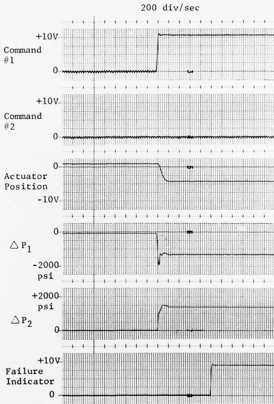
FIGURE 100  $\Delta P$  Failure Detection, 80 samples/sec.
