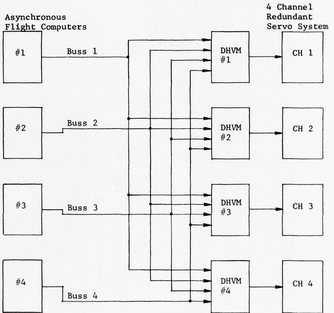
FIGURE 2 The DHVM as an element in a Digital Flight Control System
