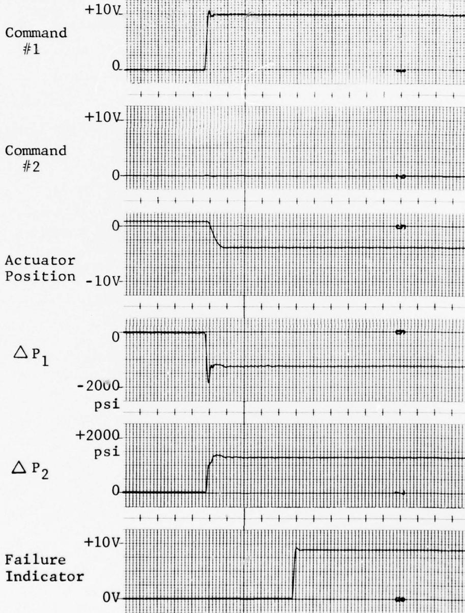
FIGURE 96  $\Delta P$  Failure Detection, Base Line
