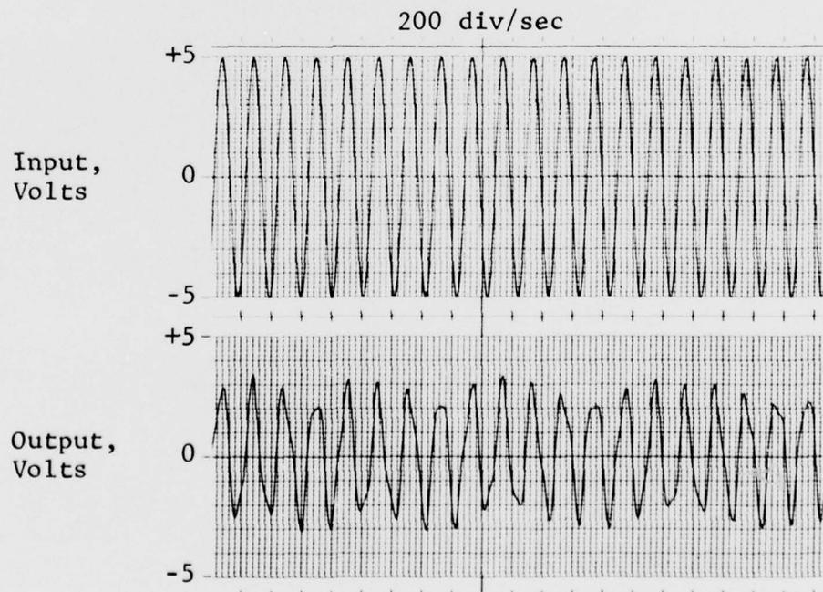
FIGURE 53 40 Hz Input-Output at 125 samples/sec.
