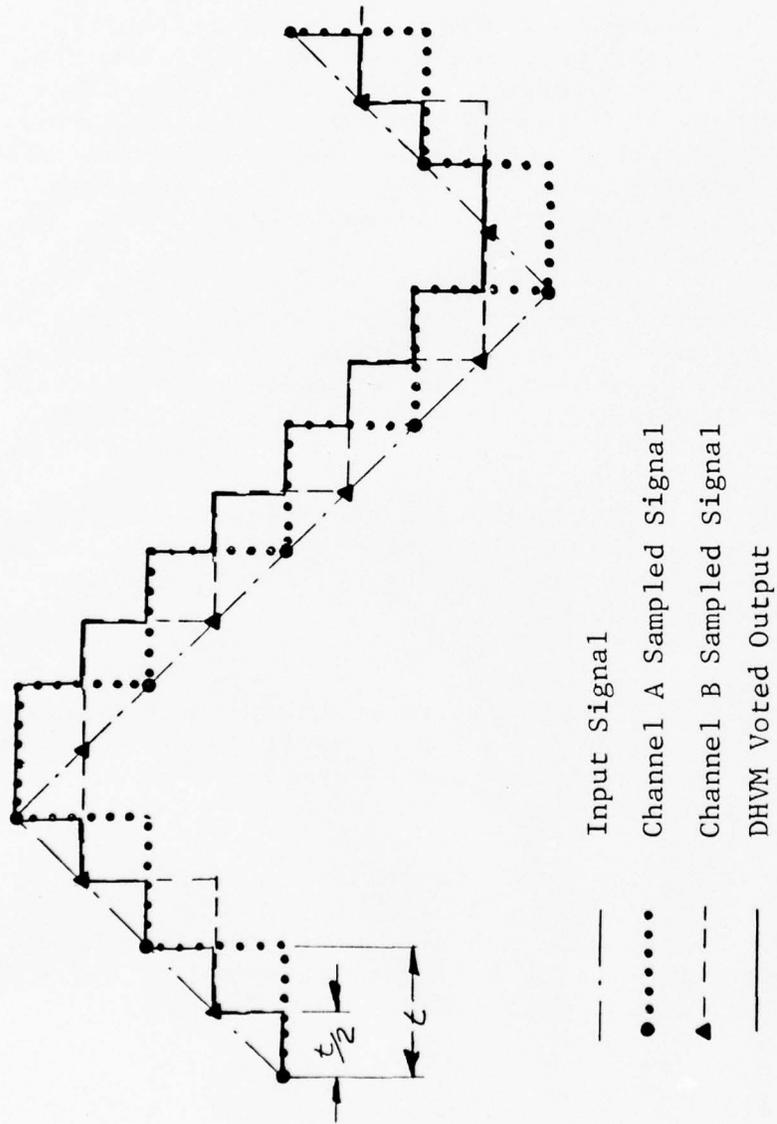
FIGURE 68 Asynchronous Sampling, with Channel B delayed by  $1/2$  of the Sample Period,  $t$ .
