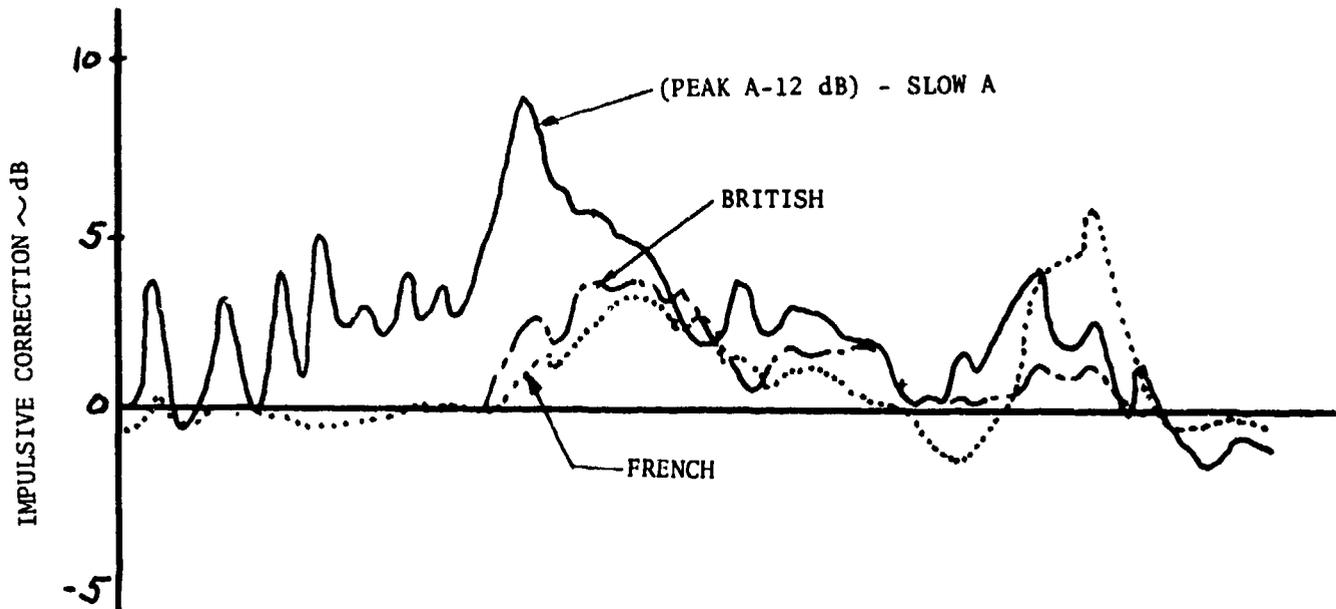
FIGURE 108 IMPULSIVE CORRECTIONS FOR CH-47C, 141KT
