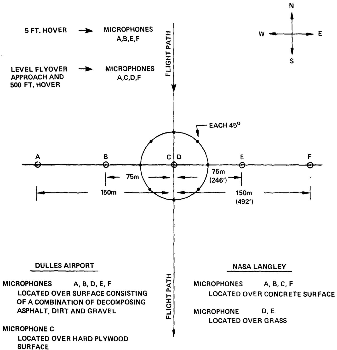
Figure 18. MICROPHONE ARRAY FOR HELICOPTER NOISE TEST.
