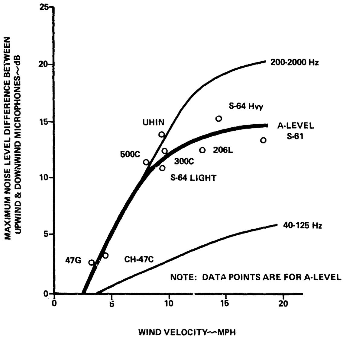
FIGURE 67. CORRELATION OF HOVER NOISE LEVEL ASSYMETRY WITH WIND VELOCITY.
