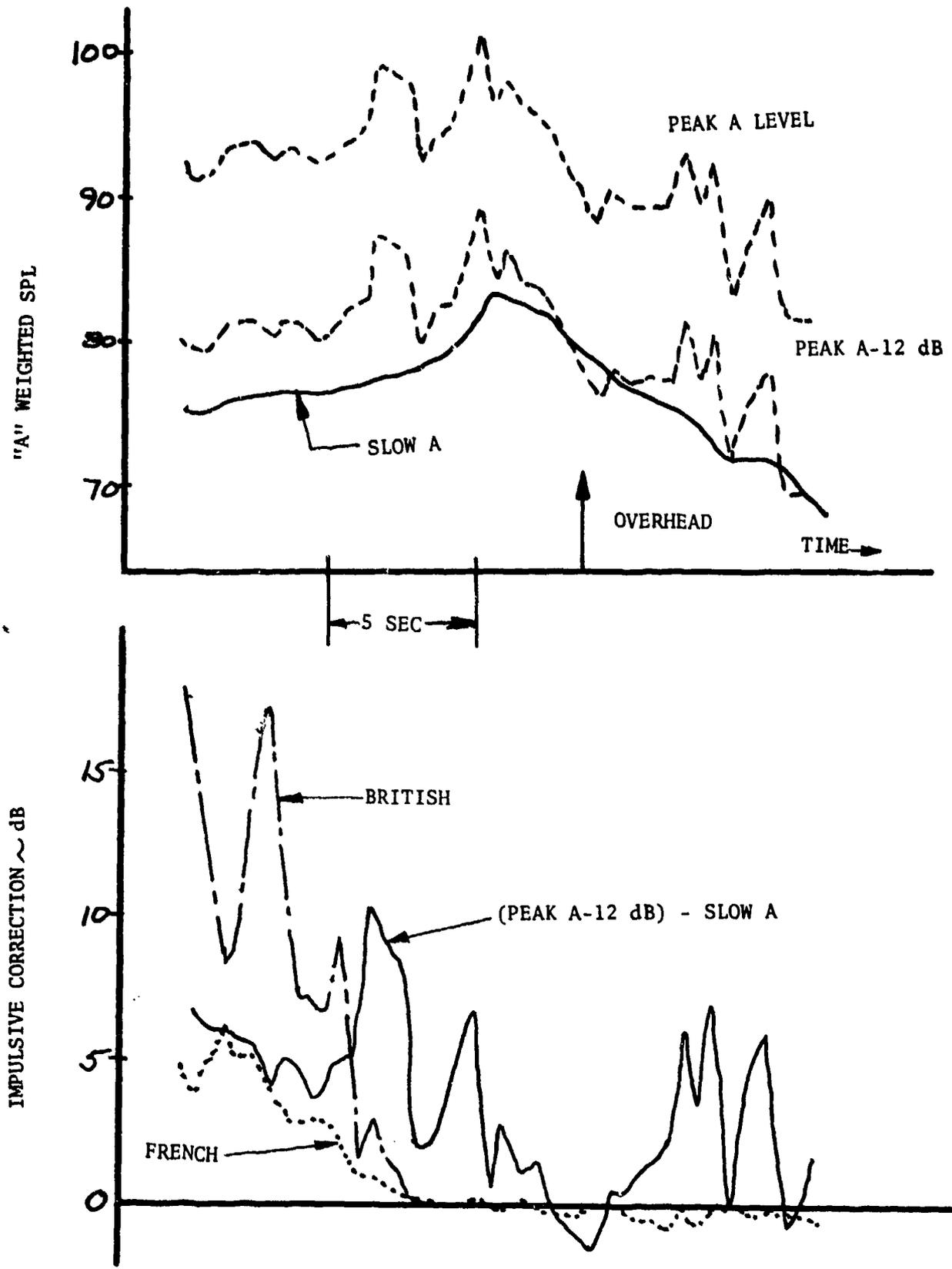
FIGURE 111 IMPULSIVE CORRECTIONS FOR UHIN, 110KT
