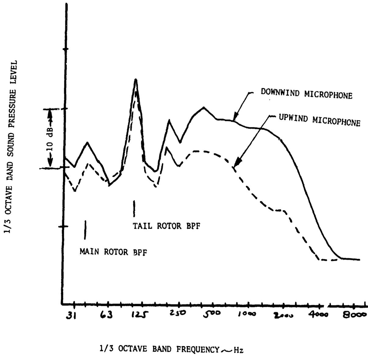
FIGURE 66. SPECTRAL CHARACTERISTICS OF HOVER NOISE ASSYMETRY
