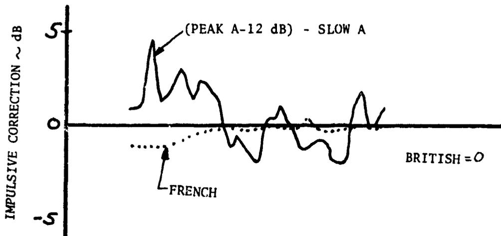
FIGURE 109 IMPULSIVE CORRECTIONS FOR S-64, 95KT
