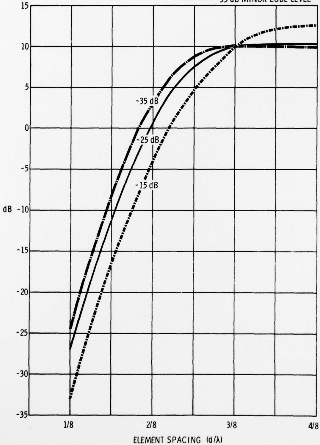
Figure 13. Signal gain (dB re single element) vs spacing and shading.
