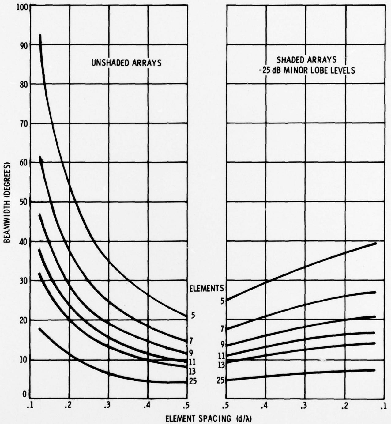
Figure 4. Beamwidth at -3 dB level.
