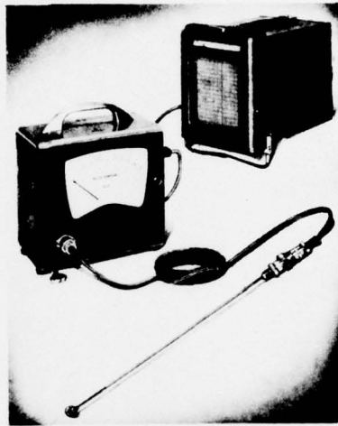
26. Miniature propeller current meters (with 4, 10 and 20-mm rotors) have been developed by the Station's instrument engineers to fulfil a need for a sensitive current meter causing minimum interference to flow patterns. The instrument will measure velocities down to about 0.7 in/sec.
