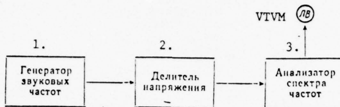
Figure 70. Circuit for calibrating a frequency spectrum analyzer.
