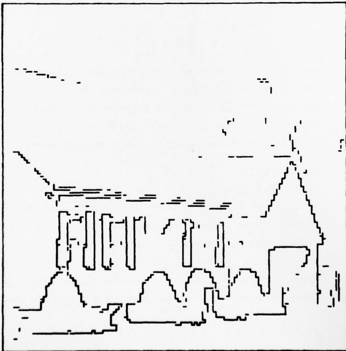
Figure 21b. Differentiated version of 21a. Edge strengths have been thresholded at .25 for display purposes only.
