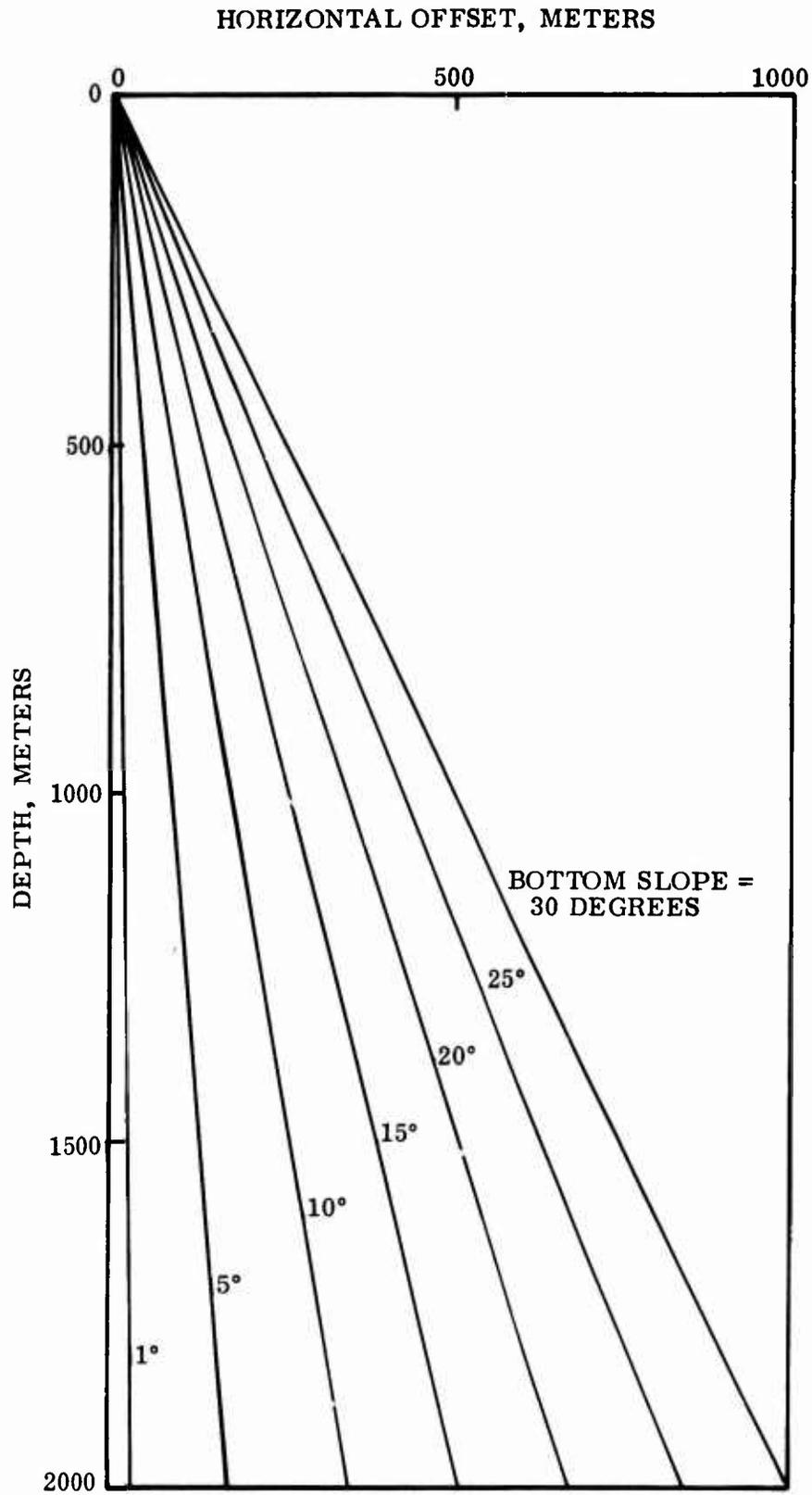
Figure 14 Horizontal Offset of Sounded Bottom with Respect to Surface Ship, as a Function of Depth and Bottom Slope, for Wide-Beam Echo Sounder.
