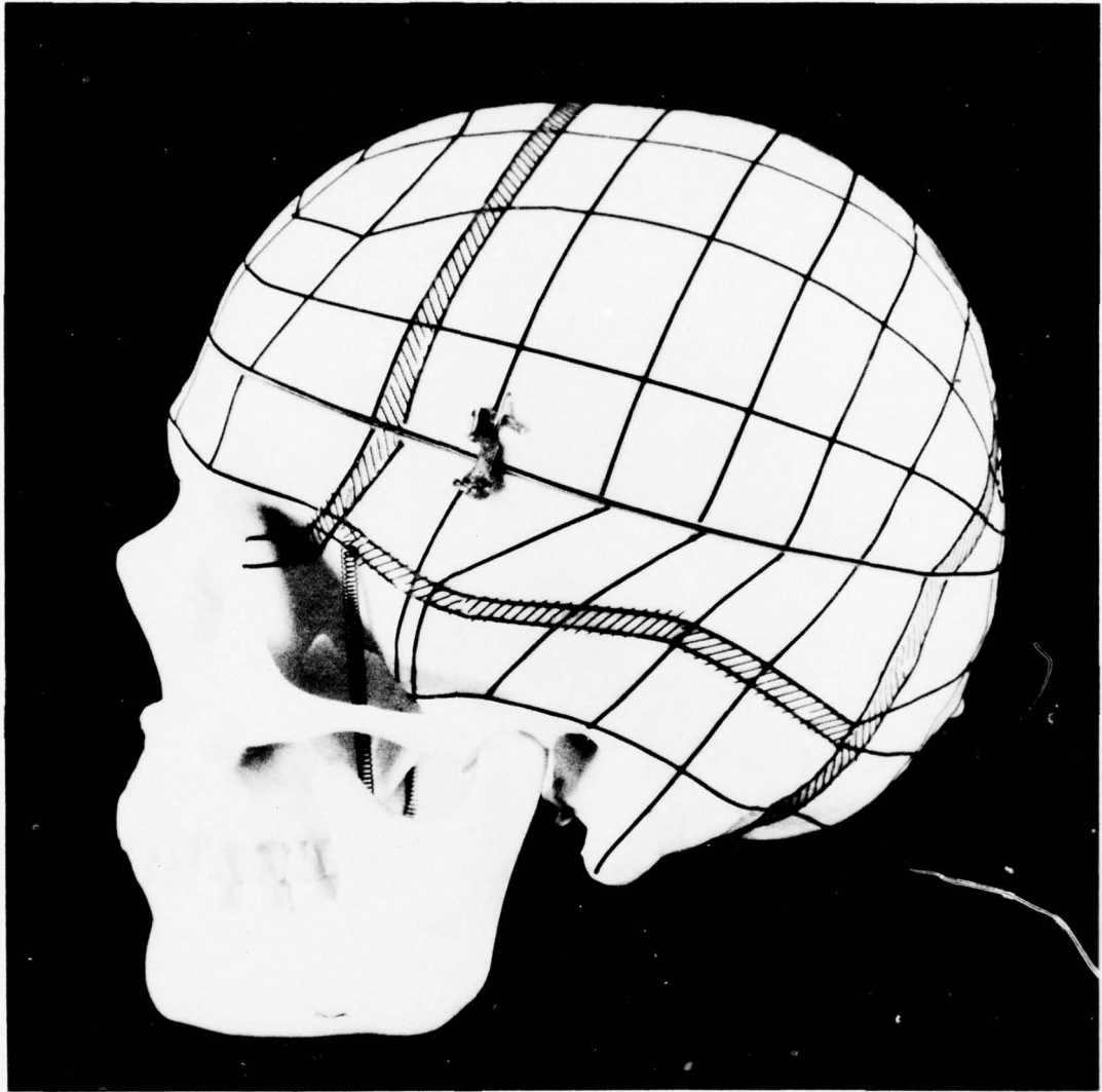
Figure 5-3. Trial Discretization of the Skull Surface Including Suture Elements.
