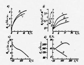
Fig. IV.23. Mechanical properties of monofils of heat-resistant polyamide "Nomex:" a - curves of stress  $\sigma$  vs elongation  $\delta$  at 21°C and various deformation rates.
