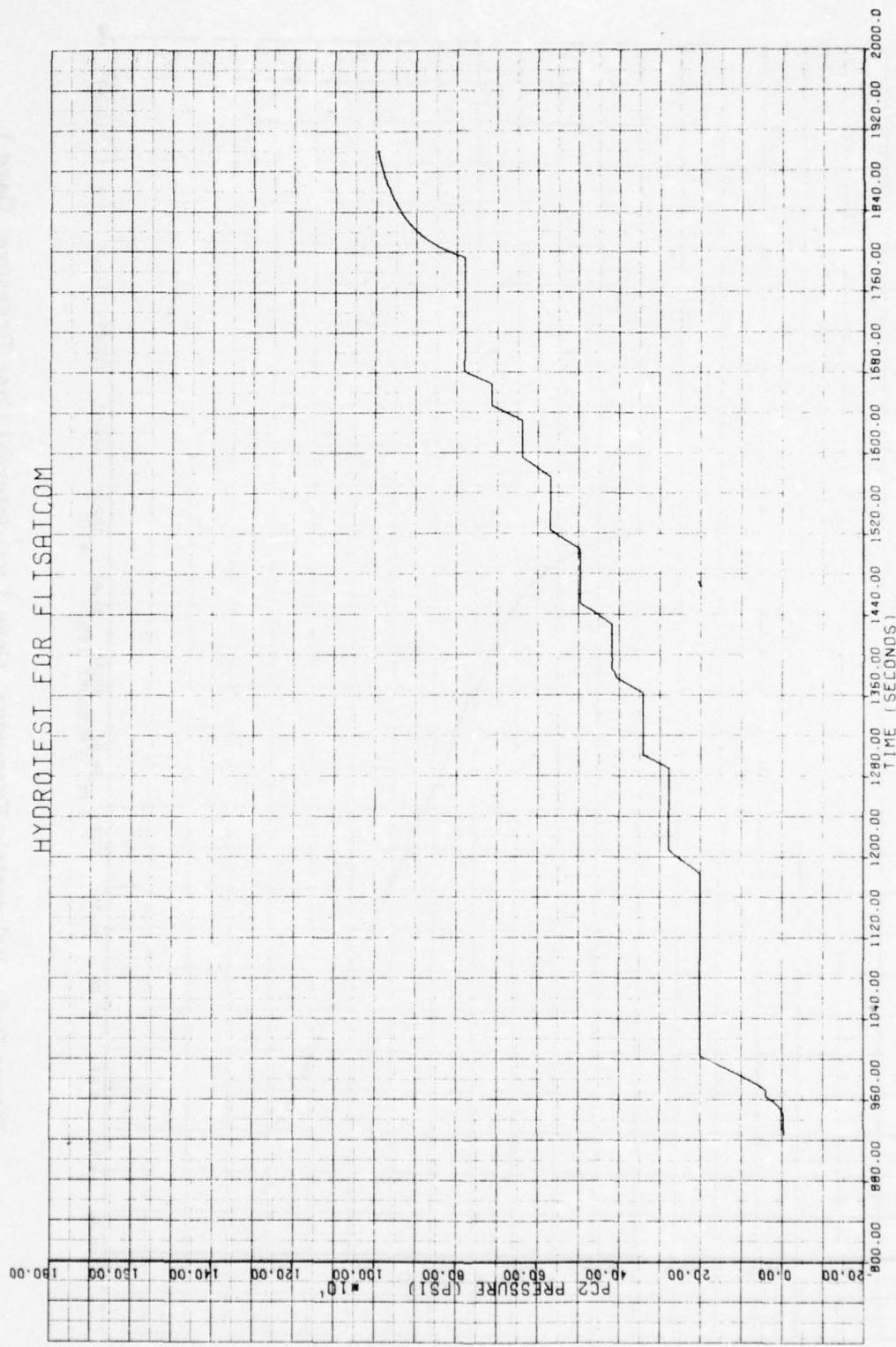
Figure B-4. Internal Case Pressure Profile, Gage 2
