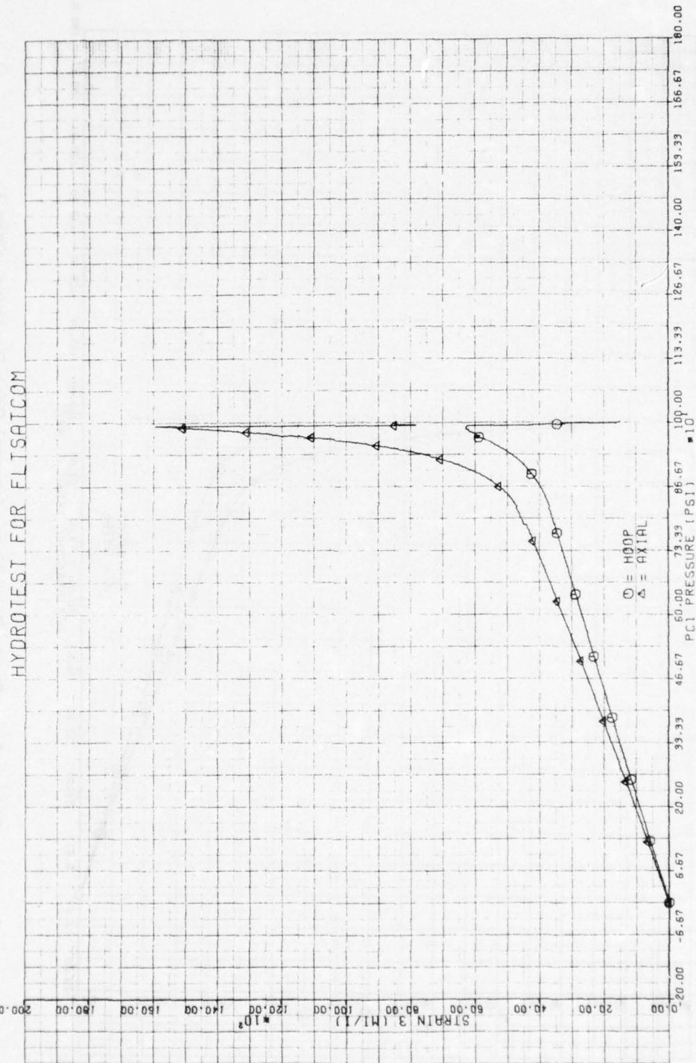
Figure C-5. Strain Gage #3 vs. Internal Case Pressure, Gage 1
