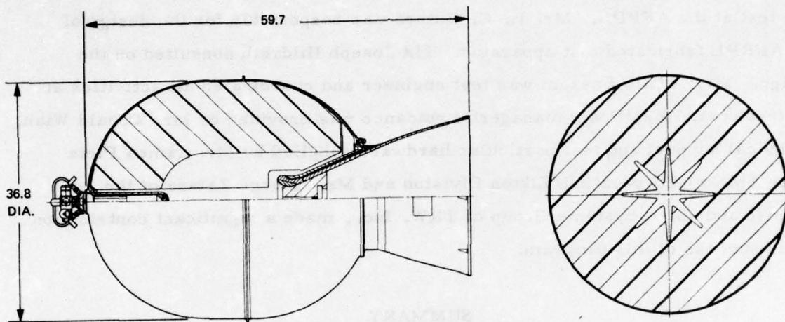
Figure 1. TE-M-364-19 Apogee Kick Motor for FLTSATCOM
