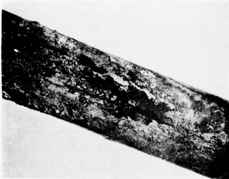
Figure 8. Corrosion attack into the interior of an AISI 430 stainless steel specimen. Only a thin uncorroded outer layer remains. (Block 45)(7.5x)
