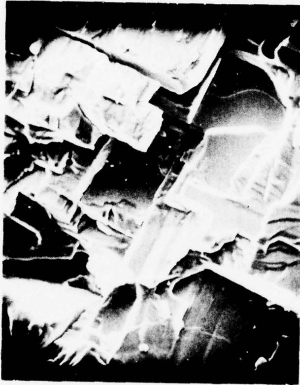
Figure II-13. Scanning electron microscope photograph of details of the damage produced by the impact of a laser pulse well above the threshold for damage on a potassium chloride target. Magnification is 500X.
