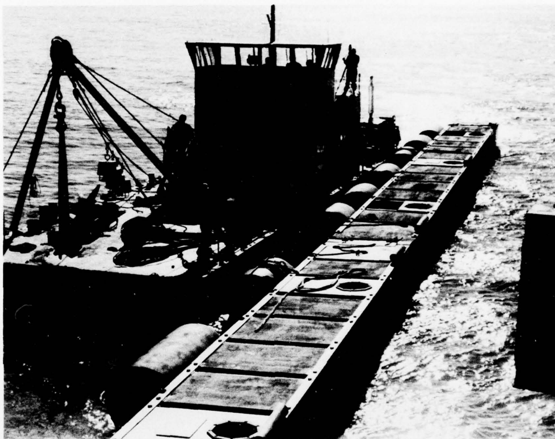
Figure 1-11. PHIBCB-ONE warping tug with fender in tow approaches elevated causeway — 24 November 1975.
