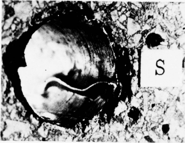
(a) STATIC LOADING (SI-35) P_{MAX} = 20,000 psi AVG. \Delta D/D = 8\%
