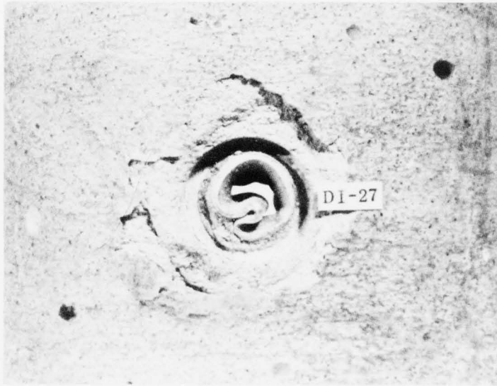
FIGURE 5-9 RESPONSE OF AN ALUMINUM-LINED TUNNEL IN HARM GROUT (CASES MODEL) TO DYNAMIC, ISOTROPIC LOADING— a/h = 6.0 , P_{\text{omax}} = 11,200 psi
