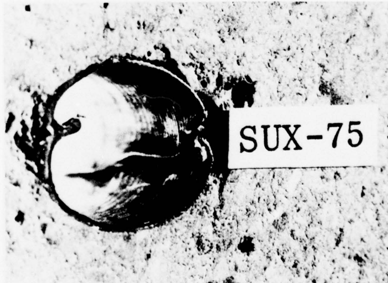
FIGURE 6-8 RESPONSE OF A STEEL-LINED TUNNEL IN DRY ROCK TO STATIC, UNIAXIAL STRAIN LOADING— a/h = 50 , P_{Vmax} = 23,500 psi, \Delta D_V/D = 0.175
