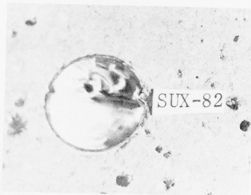
FIGURE 6-3 RESPONSE OF A STEEL-LINED TUNNEL IN SATURATED ROCK TO STATIC, UNIAXIAL STRAIN LOADING — a/h = 25 , P_{Vmax} = 19,000 psi, \Delta D_V/D = 0.147
