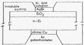
The analysis of over 200 preparations of these devices has shown them to provide stable, rapid-response potentiometric relationships for component ion activities in aqueous solutions, referenced to a saturated calomel electrode.
