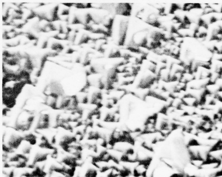
Figure 73. Surface Structure of Lithium when Stored in 1.0M \text{LiAlCl}_4 (Fused) \cdot \text{SOCl}_2 + 5% by Weight \text{SO}_2 at 162^\circ\text{F} for One Week SEM SECONDARY MODE
