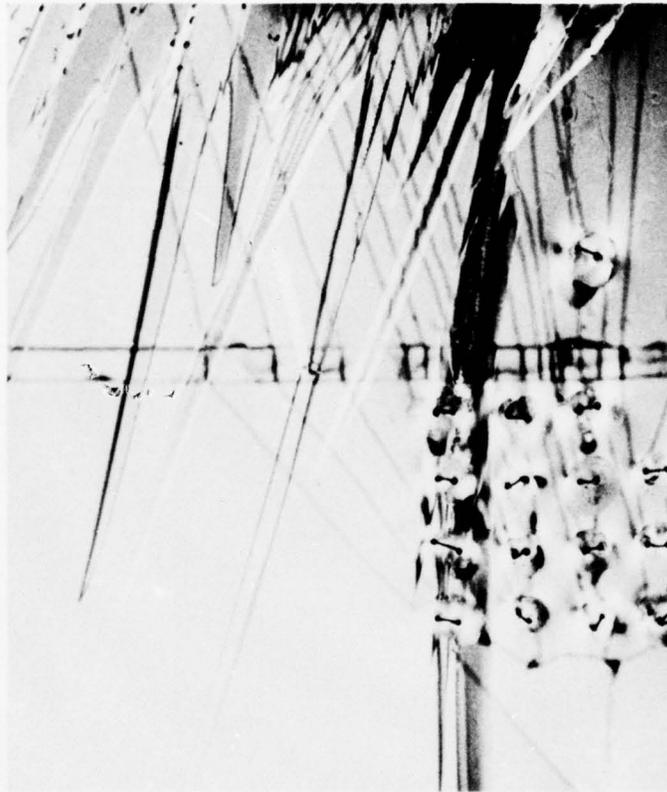
FIGURE 5. Photograph of tank with ice crystals that formed from supercooled water. The square array has 15 thermocouples separated by 5 mm. In the background is a horizontal plastic spacer for the thermocouple wires.
