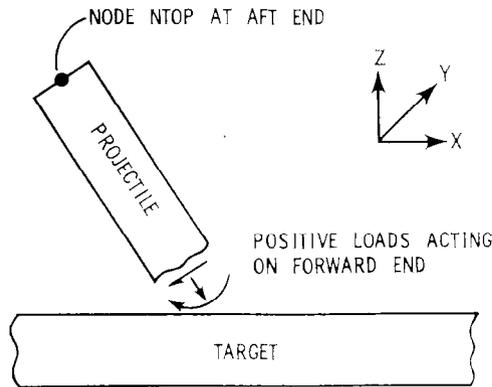
Figure 18. Sign Convention for Internal Projectile Loads
