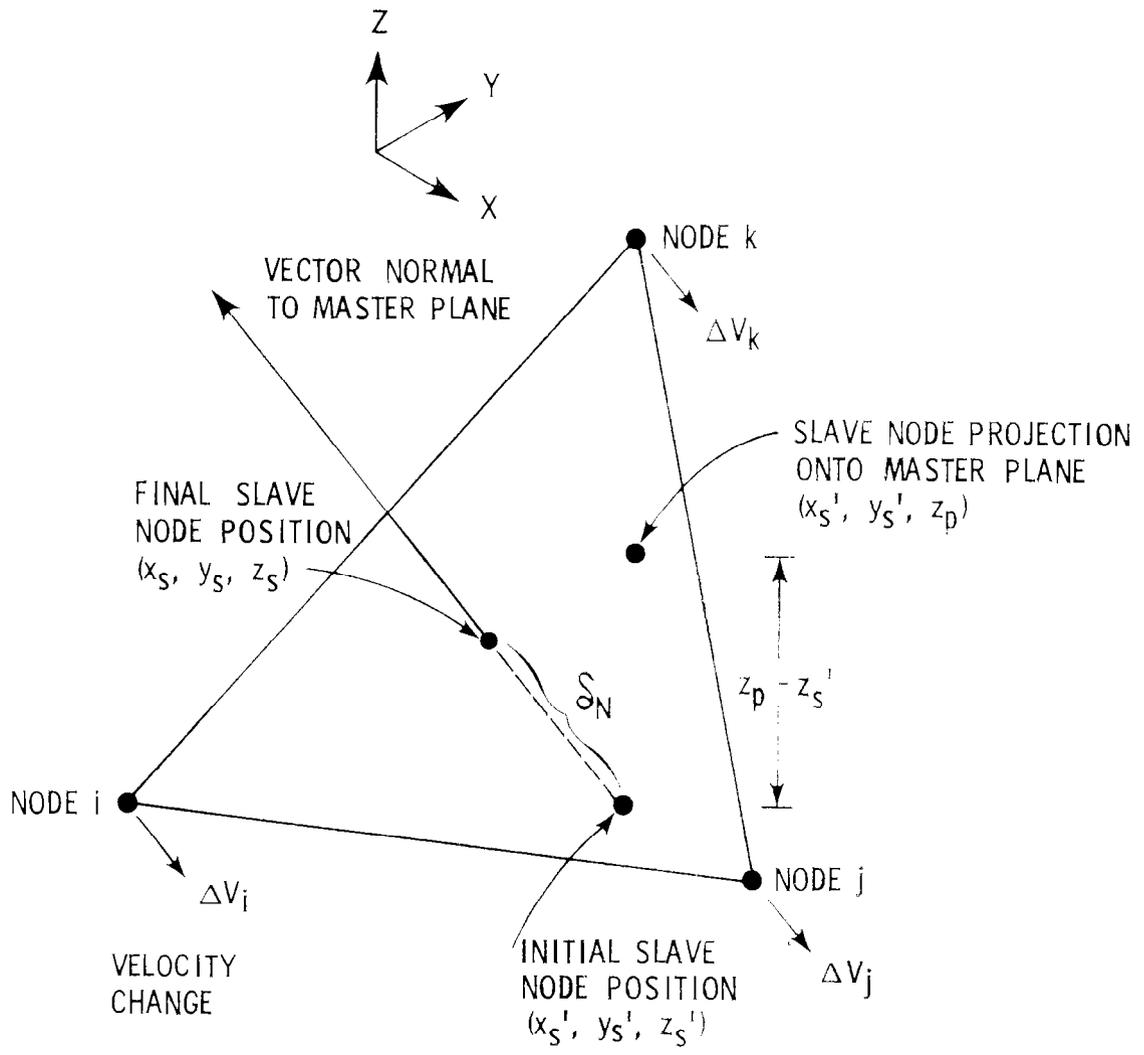
Figure 4. Slave Node Placement onto Master Surface
