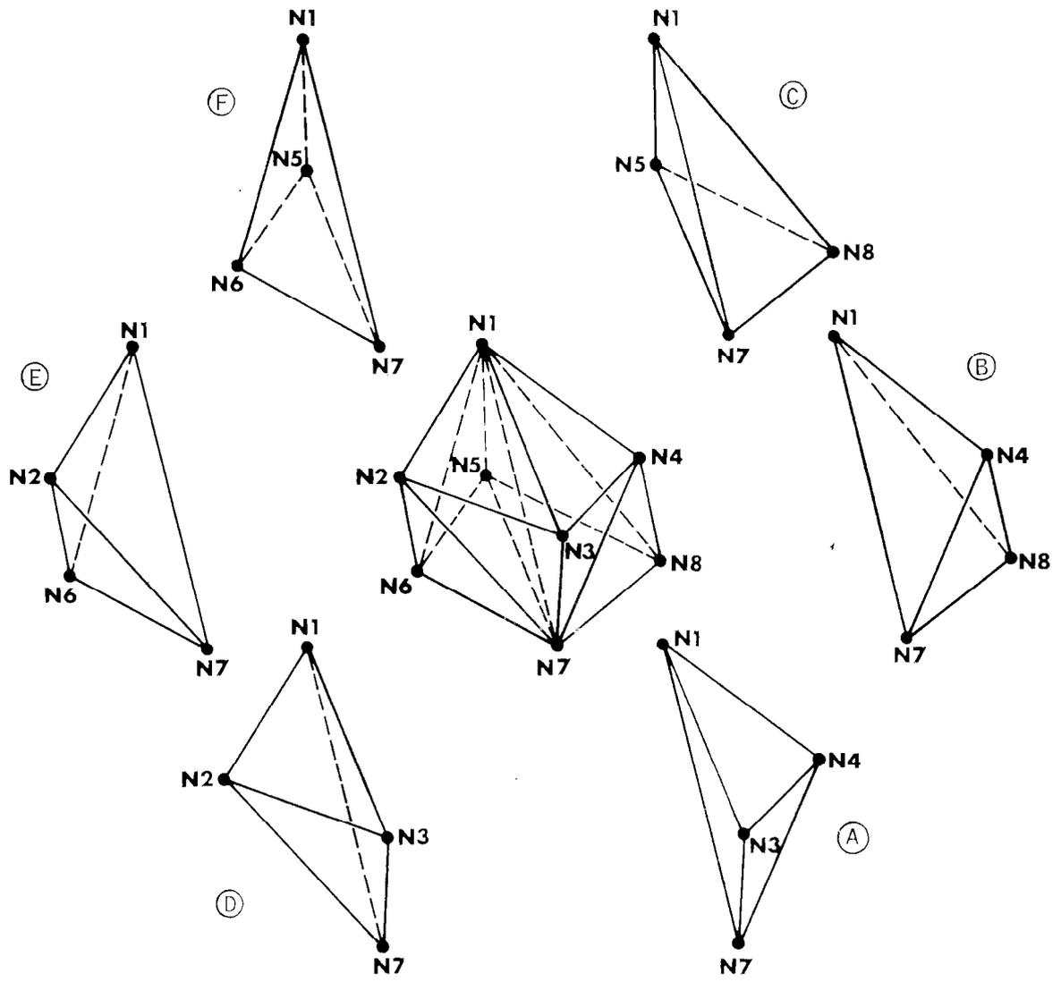
Figure 8. Arrangement of Six Tetrahedra into a Composite Brick Element
