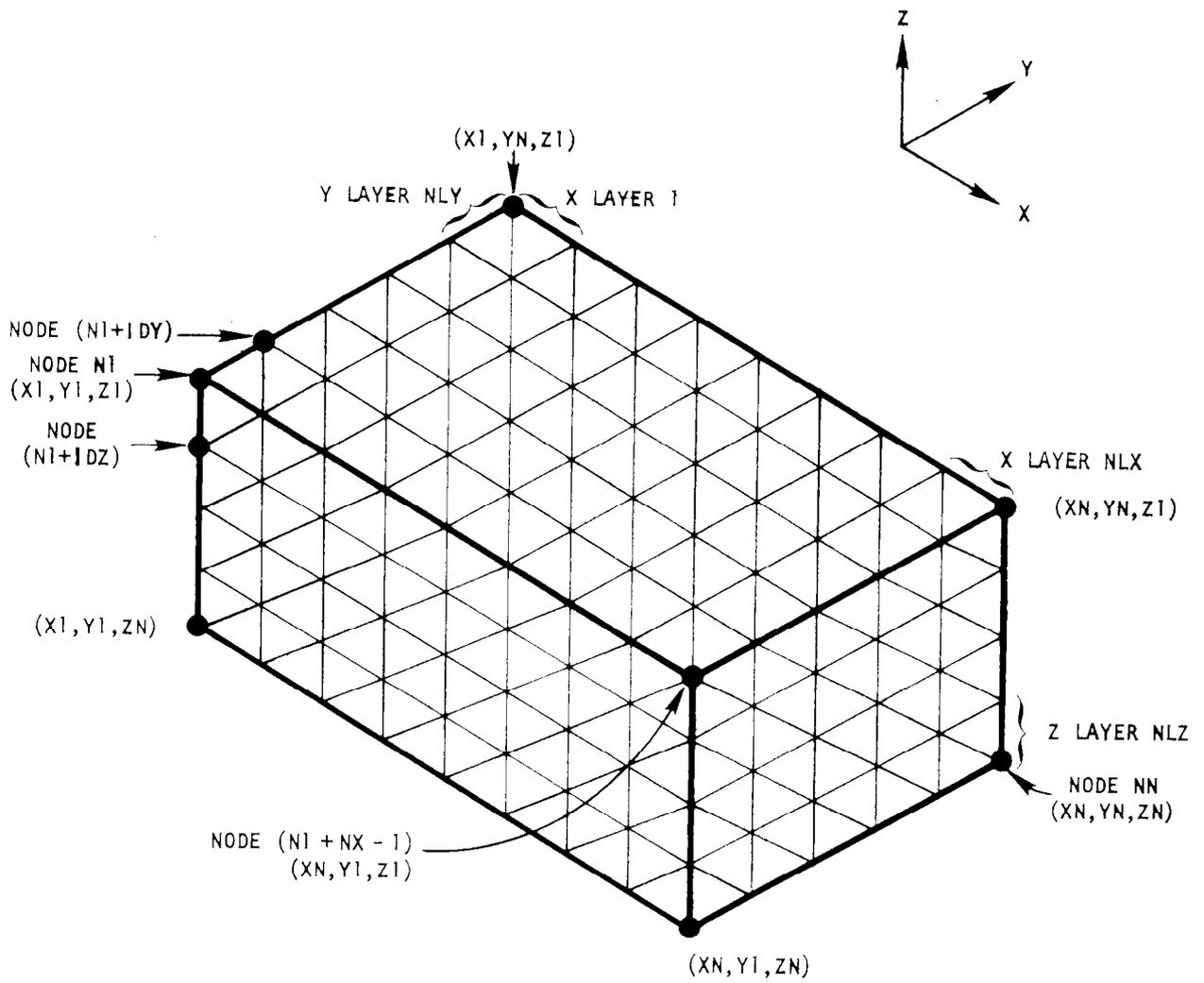
Figure 15. Geometry of Special Plate Shapes
