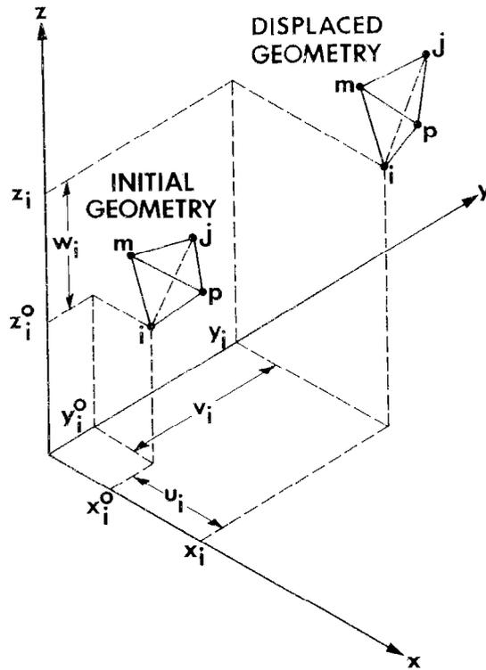
Figure 2. Geometric Properties of a Tetrahedron Element
