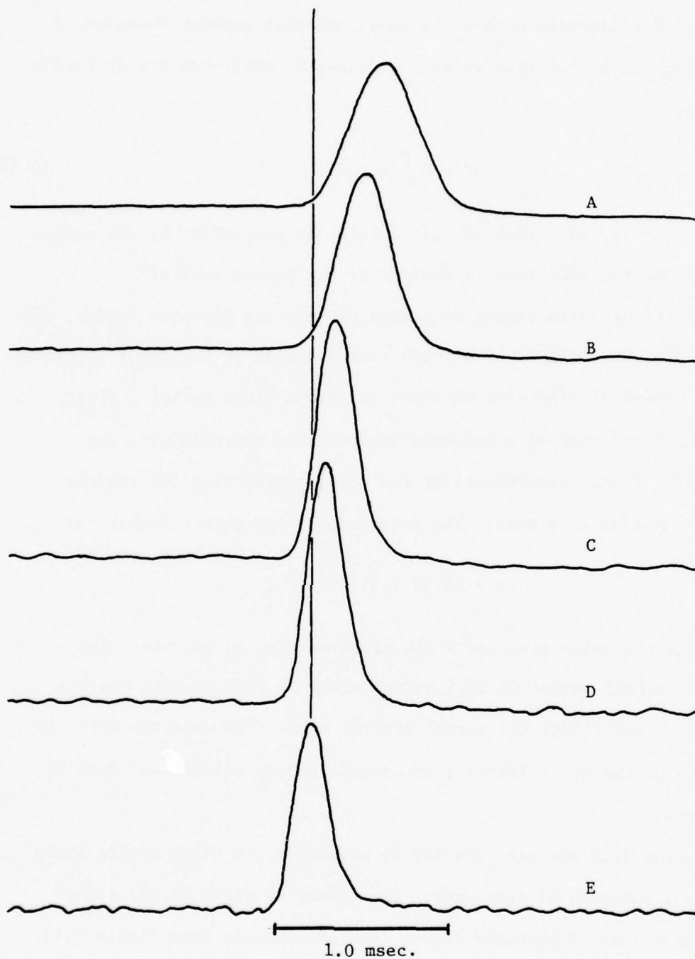
Figure 5.15. Pulse delay and spreading after transversal filtering. Clock frequency for: A = 46 kHz; B = 65 kHz; C = 189 kHz; and D = 543 kHz. E is unfiltered. Gain settings for A-D are the same.
