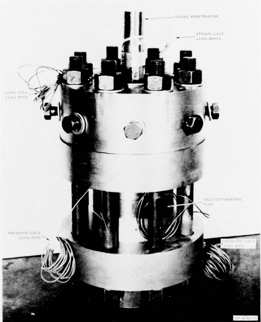
FIGURE 4 ASSEMBLED TEST FIXTURE FOR SIMULATING IMPACT LOADS
