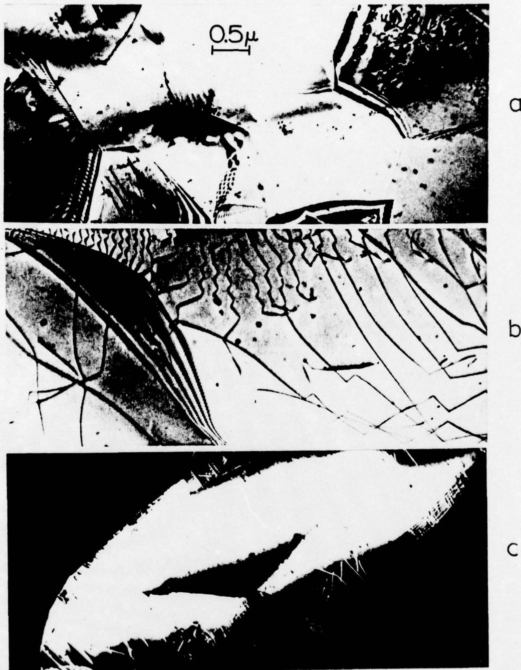
Fig. 7. Beryllium sheet structure observed in the transmission electron microscope. (a) Small-grained structure of commercially sintered-rolled beryllium sheet. (b) Dislocation networks in annealed sheet Be. (c) Dark-field image showing grain boundary defect structure in annealed Be sheet.
