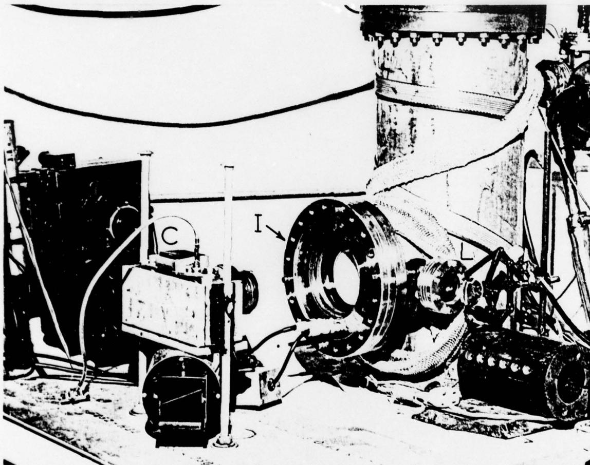
Fig. 3. Field-ion microscope showing channel-plate (imaging screen) (I), laser thru-port (L), and camera (C).
