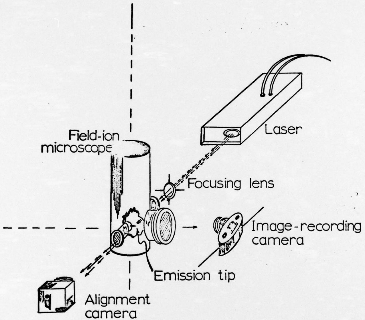
Fig. 1. Field-ion microscope in-situ irradiation system (schematic).
