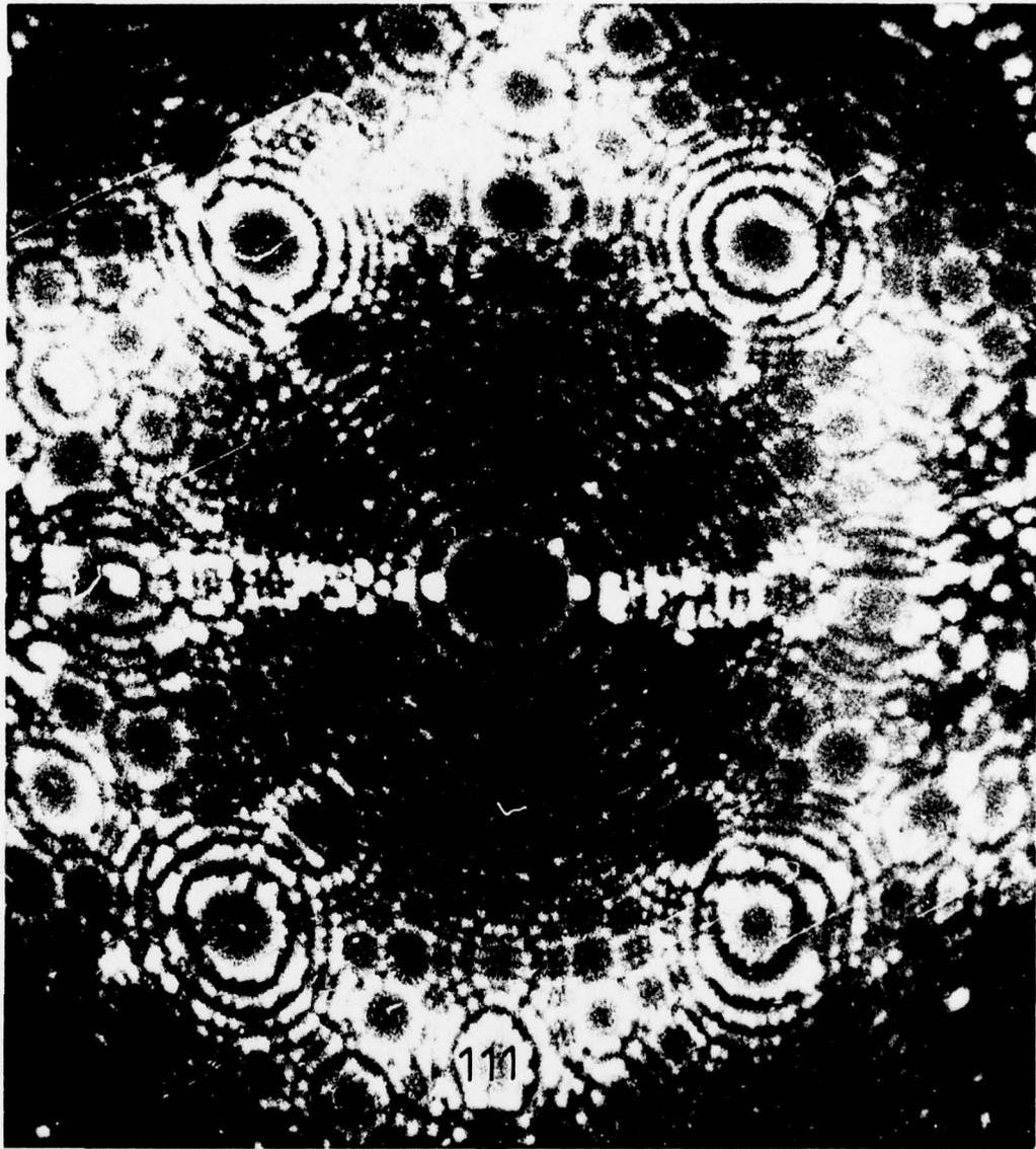
Fig. 10. Tungsten field-ion image showing end-form surface as viewed in the field-ion microscope.
