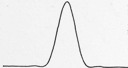
Fig.1. a) Mode intensity distribution for a Voigt profile using measured linewidth data and known cavity loss.
