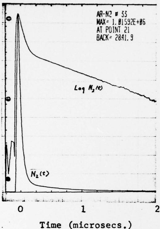
Fig.4.  $N_2 C^3P_u (v'=0)$  as function of time (from  $\lambda 3371 \text{ \AA}$ ) after threshold energy electron pulse for  $Ar(3P_2)$  metastable is turned off in  $Ar - N_2$  mixture. (Ar at 1.66 Torr and  $N_2$  at 1.8 Torr at 663  $^{\circ}K$ .)
