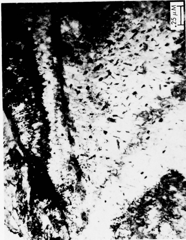
INTERLATH CEMENTITE PLATELETS AND SPHERIODIZED PARTICLES
