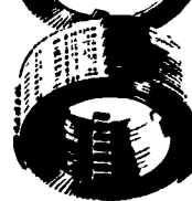
Balance Of Inner And Outer Discs With Separator Springs
