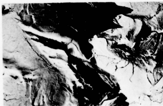
FIGURE 9. Quasi-cleavage SCC facets in precipitation hardening steel. Replication electron fractograph, magnification 2400X. Courtesy of Mr. D. A. Meyn.
