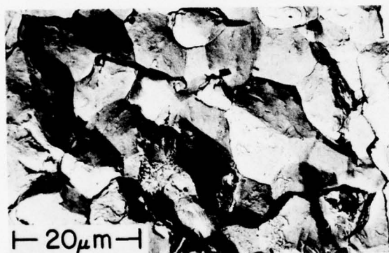
FIGURE 8. Intergranular SCC in martensitic steel. Replication electron fractograph, magnification 2250X. Courtesy of Mr. C. D. Beachem.
