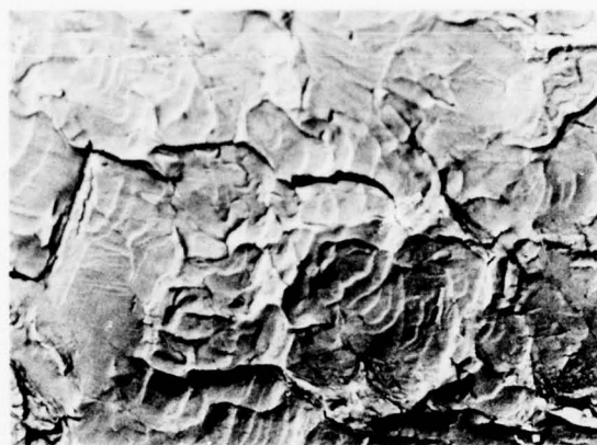
FIGURE 9. Terraced Cleavage in Ti-8%Al-1%Mo-1%V cracked in gaseous hydrogen. Electron fractograph, magnification 3000X. Courtesy of Mr. D. A. Meyn.
