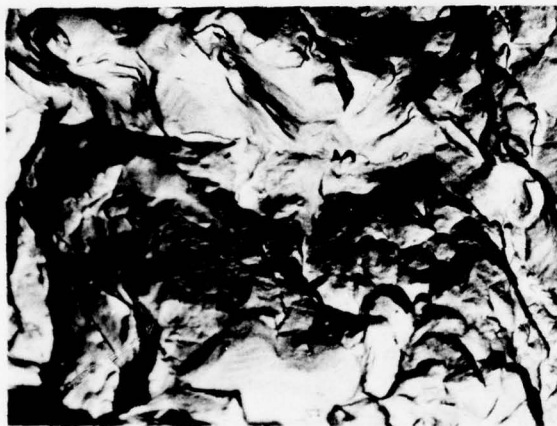
FIGURE 6. Dimples of variegated size produced by purely mechanical "plane strain" fracturing of Ti-8%Al-1%Mo-1%V. Electron fractograph, magnification 6000X. Courtesy of Mr. D. A. Meyn.
