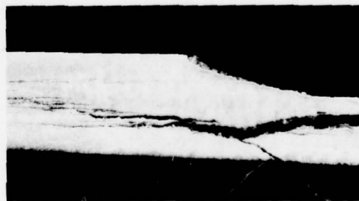
FIGURE 10. Intergranular stress corrosion cracks in alloy 5456, showing extensive branching. Optical micrograph of polished section, magnified 7X. Photo courtesy of Dr. C. T. Fujii.
