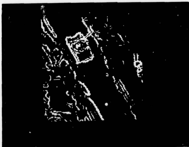
Modified gradient picture of target (tank) region in Fig. 1 on noise cleaned data. Threshold is 35.
